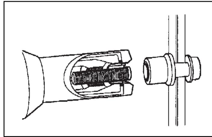
Figure 2.12 Body of Fastener Separates at Breakneck 01\_0022
