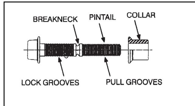
Figure 2.7 Huckbolt Fasteners
