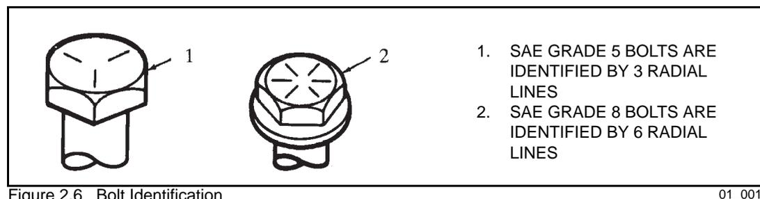
These bolts, 0.5 inch (13 mm) diameter flange head type, should be tightened to 110 to 120 ft-lbs. (149 to 163 Nm) based on new bolts and nuts lubricated with engine oil. Whenever possible, hold the bolt and tighten the nut.
