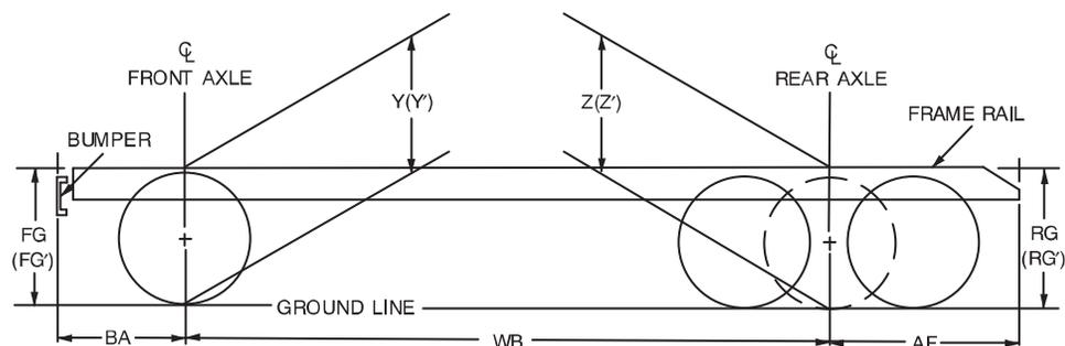
FIRST WE MUST DETERMINE THE RAKE OF THE FRAME (I.E., THE SLOPE OF THE FRAME FROM FRONT END TO REAR END). IF THE FRONT END OF THE FRAME IS HIGHER THAN THE REAR END (I.E.,  $Y > Z$  OR  $Y' > Z'$ ) THEN THE TRUCK IS SAID TO HAVE A NEGATIVE RAKE. IN THIS SITUATION, THE EQUATIONS FOR DETERMINING THE FRAME HEIGHT AT THE RAIL ENDS ARE:
