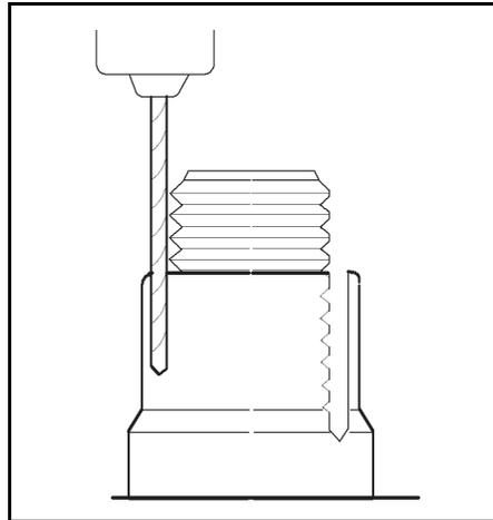
Figure 2.15 Drilling
