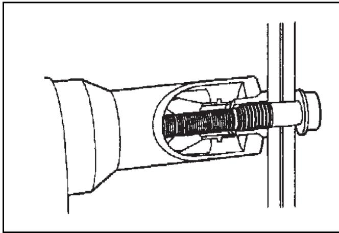
Figure 2.11 Clamping Force is Developed 01\_0021
