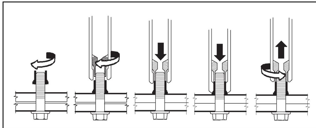
Figure 2.20 Huck-Spin Installation 01\_0030
