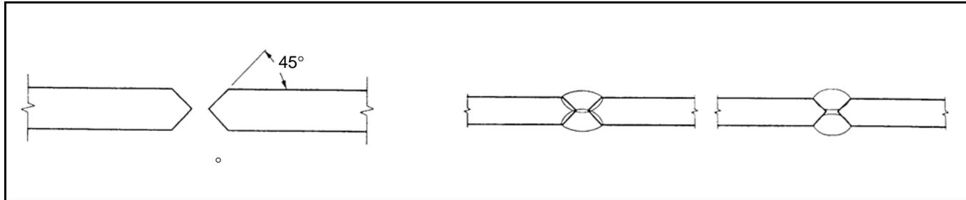
Figure 2.24 Frames – Preparation of Joint for Welding Extension
