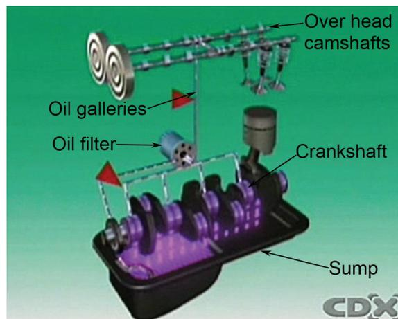
The galleries allow oil to be fed to the camshaft bearings, the valve mechanism and the crankshaft main bearings. Holes drilled in the crankshaft webs allow the main bearings to supply oil to the big-end bearings.
