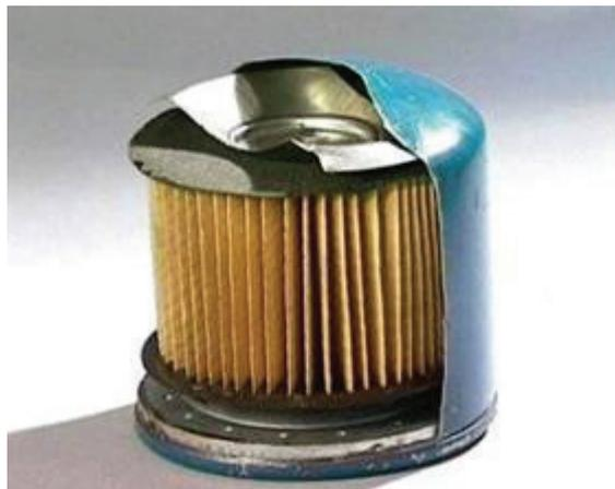
Normally all oil goes through the filter before it gets to the engine, but if the filter clogs up, it can starve an engine of oil. As a safety measure, full-flow filters have a bypass valve. If the filter clogs, this valve opens and directs unfiltered oil to the engine. Dirty oil is better than none at all.
