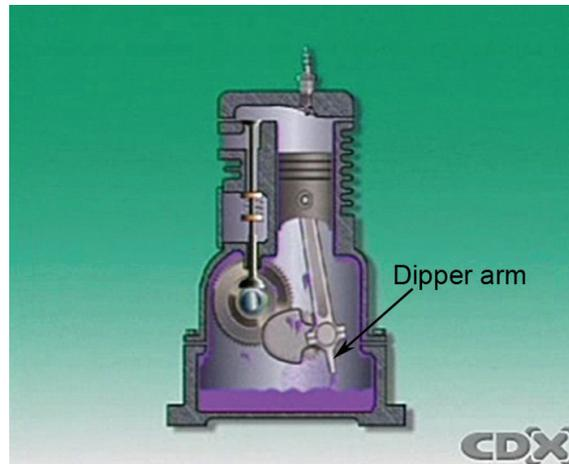
On horizontal-crankshaft engines, a dipper on the bottom of the connecting rod scoops up oil from the crankcase for the bearings. In this engine it is also able to splash oil up to the valve mechanism.
