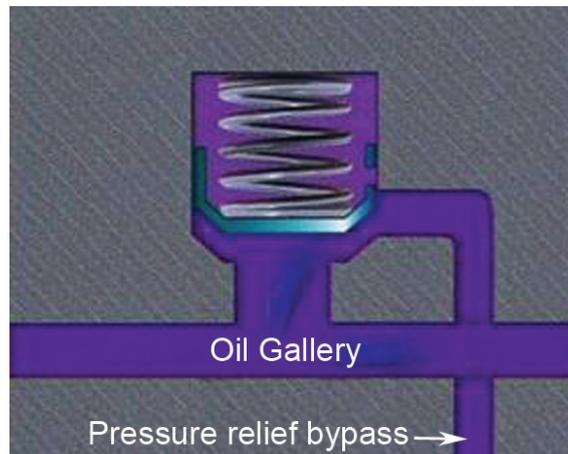
A normal pump is capable of delivering more oil than an engine needs. It's a safety measure to ensure the engine is never starved for oil. As the pump rotates and engine speed increases, the volume of oil delivered also increases. The fixed clearances between the moving parts of the engine prevent oil escaping back to the sump and pressure builds up in the system.
