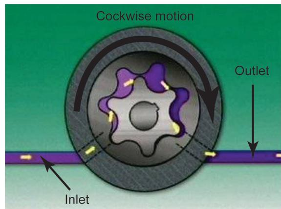
In a *rotor-type oil pump*, an inner rotor drives an outer one. This is generally driven by the camshaft. As they turn, the volume between them increases. This larger volume lowers the pressure at the pump inlet. Outside atmospheric pressure is then higher. This forces oil
