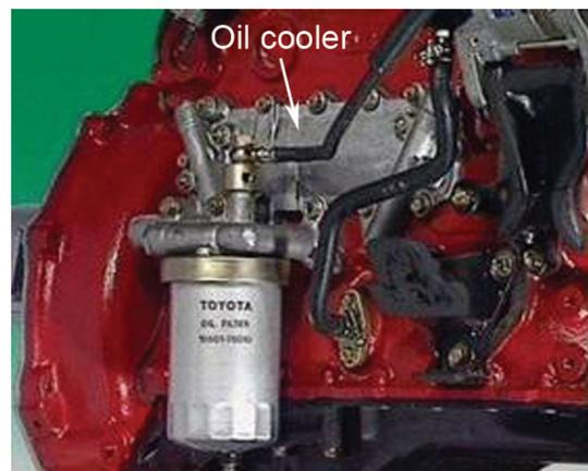
In diesel engines, the oil cooler and oil filter are often on the same mounting, on the cylinder block.
