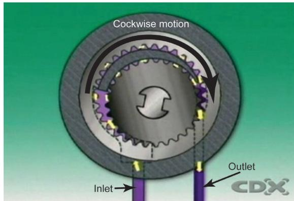
This is generally driven by the crankshaft. The inner gear is on the end of the crankshaft which then drives the pump directly. An external toothed gear meshes with this inner one. Some gear teeth are meshed but others are separated by the crescent-shaped part of the pump housing. The increasing volume between gear teeth causes pressure to fall. Oil is then taken through the intake port and carried around between the gears and crescent, then discharged to the outlet port.
