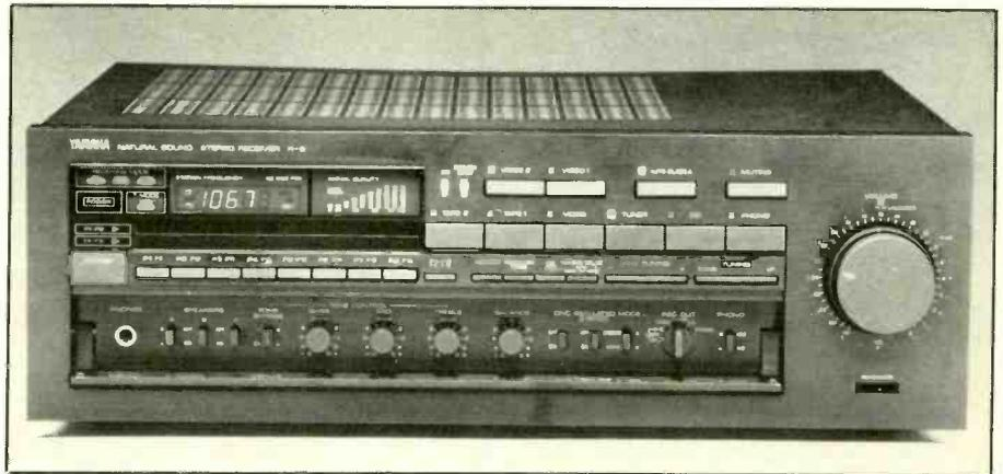
amplifier section to Class A operation. For signals requiring less than 20 watts per channel (and that's most music most of the time), the amplifier remains in Class A. For those occasional brief peaks that require more instantaneous power, the amplifier automatically reverts to Class AB.
