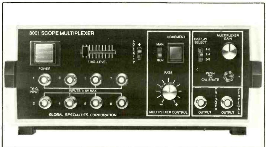
be set up to display a single waveform or, with the flip of a switch, four or eight waveforms simultaneously. Furthermore, an incrementing circuit whose function is activated with the touch of a switch lets you step through all input channels individually for examination of a single waveform at a time.
