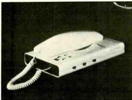
ing circuit that detects voice and data carrier and automatically passes the signal to the computer or telephone. A built-in 2" speaker lets you monitor the call, while a built-in clock/calendar feature lets you keep track of call length on your computer's video monitor screen.
