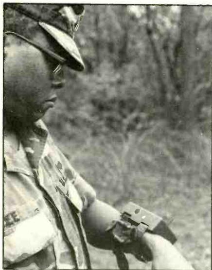
The U.S. Army continually develops new electronic equipment. Among the latest devices, reports the U.S. Army Electronics Research And Development Command, is a wrist-worn receiver for Airborne troops that works in conjunction with a small transmitter that might be carried by a paratrooper leader or packed on top of equipment to be dropped.
