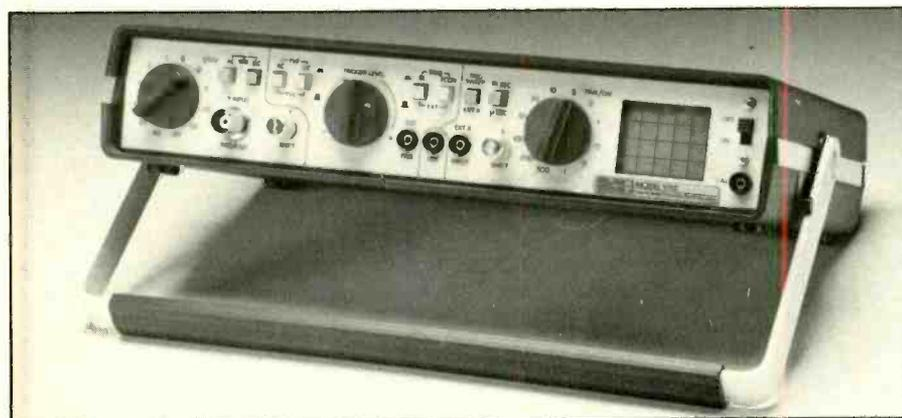
and adds only 2 lbs. to the carrying weight. The compact Model 1010 provides 12 sensitivity ranges and 21 timebase ranges. Vertical sensitivity is selectable from 10 mV/division to 50 volts/division, and timebase is variable from 0.1  $\mu$ s/division to 0.5 s/division.
