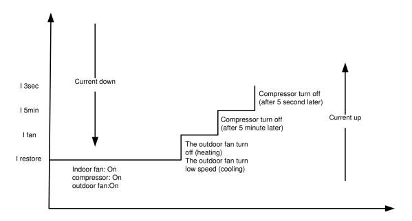
If compressor turns off for continuously 4 times due to current protection in 5 minutes from Compressor On, the unit stops and LED displays failure information and can't returns to normal operation automatically.
