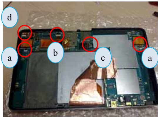
16. Connect Below FPC a. speaker FPC b. Touch panel FPC c. camera FPC d. Soft Key FPC
