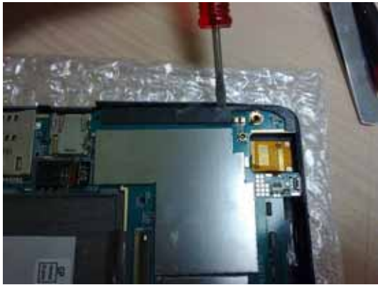
19. Use slotted screwdriver to pull the PCB board up.
