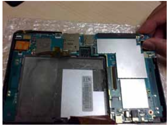
20. Pull up the PCB board carefully.
