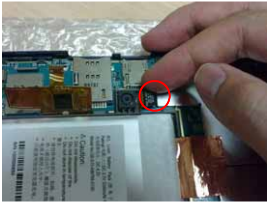
13. Release the SUB FPC BTB (Board to Board) connector.
