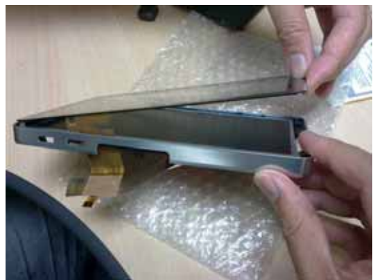
24. Remove the touch-panel from the LCM carefully, especially in FPC connector.
