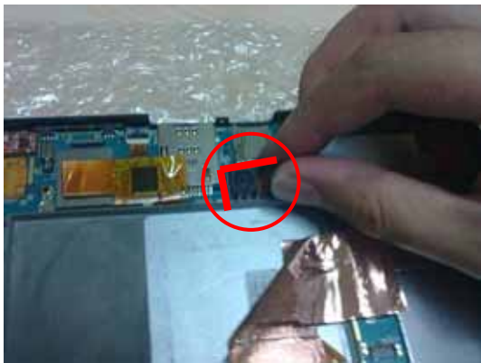
15. Assemble the camera in camera hole, according to the left & top side.
