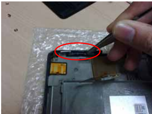
19. Use slotted screwdriver to pull the PCB board up.
