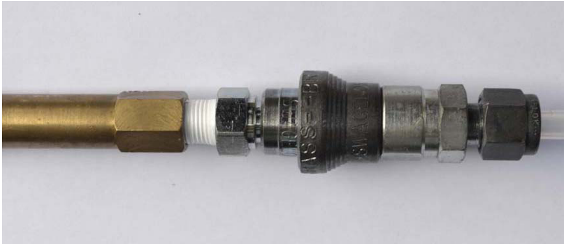
Figure 14. Assembled male fitting, female fitting and cassette extension fitting
