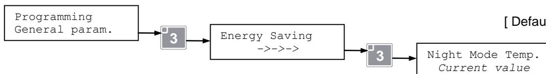
The refrigerator temperature raising function is deactivated during the **Night-Mode** period if the parameter is set to '0' (Zero) or to a value below the one set as standard internal temperature ('Set Std Temp 1' in the "Refrig. Param's" menu).
