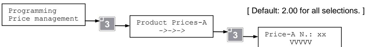
Press keys 1 and 2 to scroll through the available price lines with xx going from L01 to L041 plus S1, S2, S3, which correspond to the price lines for the direct selection buttons (max 3 optional buttons).
