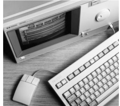
Figure 22. The 16500C's easy-to-use interface includes a touch screen, PS-2 mouse and optional keyboard.
