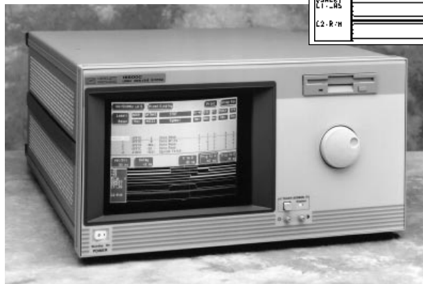
Figure 3. The HP 16500C logic analysis system can be operated using its own built-in user interface, without the HP 16505A.
