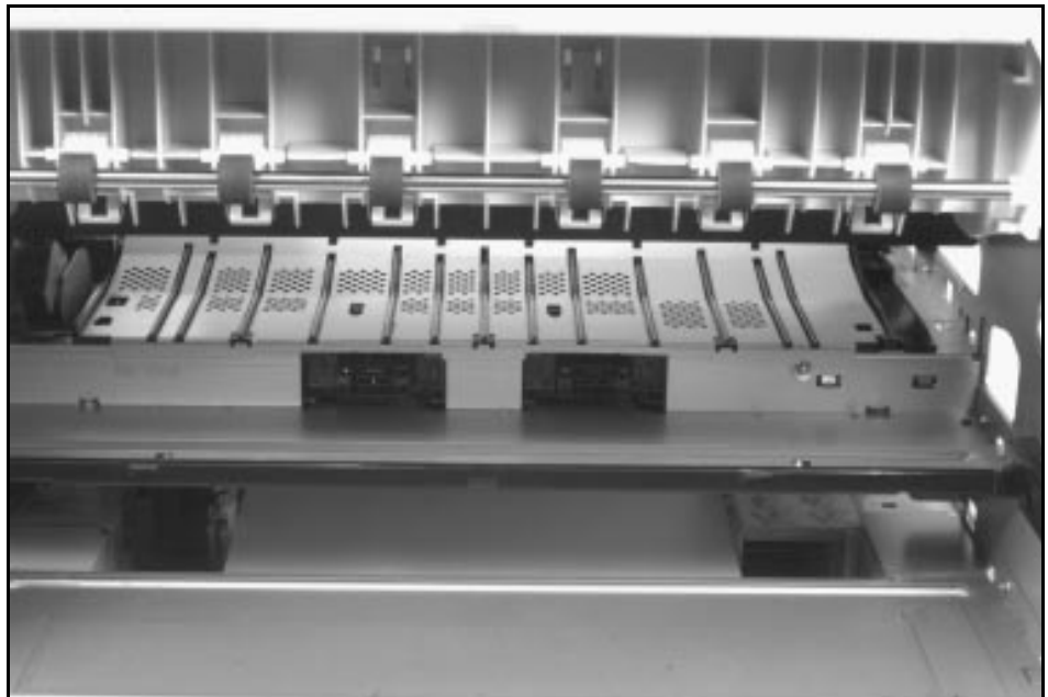
Feeder Assembly (2 of 2)
