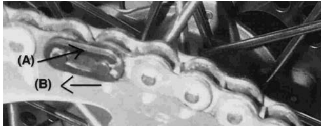
(A). Clip. (B). Direction of Chain Rotation.
