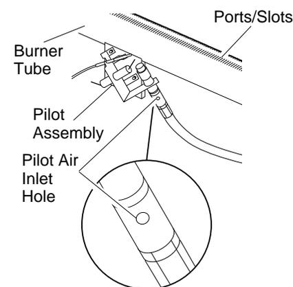
**Figure 28 - Pilot Inlet Air Hole**
