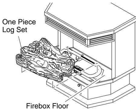
Figure 9 - Installing One-Piece Log Set
