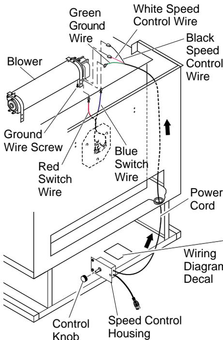
Figure 20 - Connecting Switch, Blower, and Speed Control Wires
