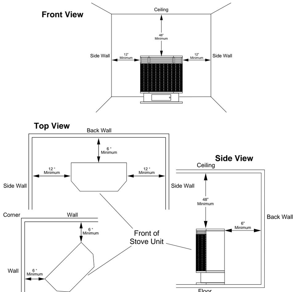
Figure 4 - Minimum Clearance to Walls and Ceiling
