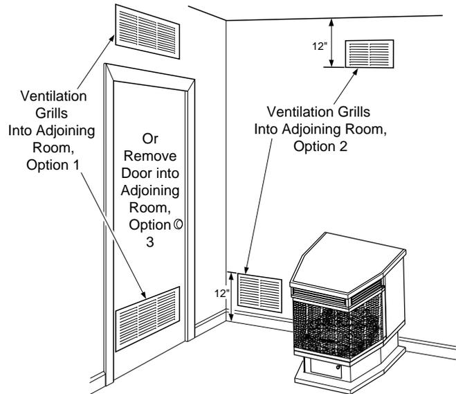
**Figure 2 - Ventilation Air from Inside Building**
