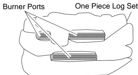
Figure 10 - Installing One-Piece Log set (Top View)
