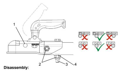
Unscrew locking nuts (2), pull out screws. Remove coupling.
