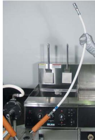
Disconnect the DRAIN HOSE and drain into WASTE OIL CONTAINER.
