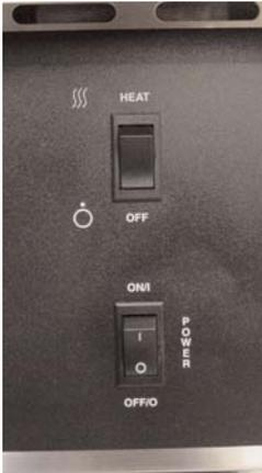
Place the **POWER SWITCH** in the **OFF** position. Turn the **HEAT SWITCH** to the **OFF** Position.
