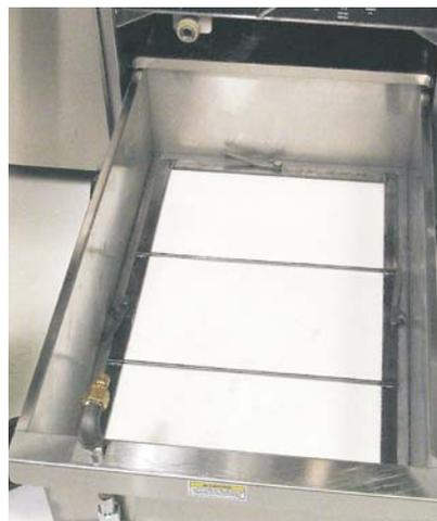
Replace the HOLD-DOWN BRACKET and **SECURELY LOCK** all 4 handles.
