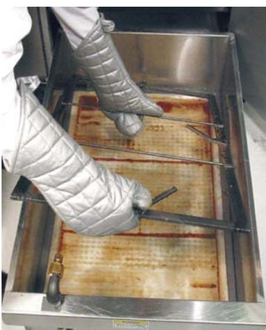
Remove the **HOLD-DOWN BRACKET** from the **FILTER PAN**.
