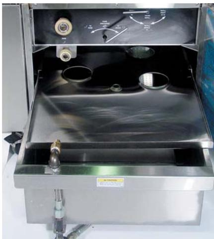
Disconnect the FILTER PAN and remove for cleaning.
