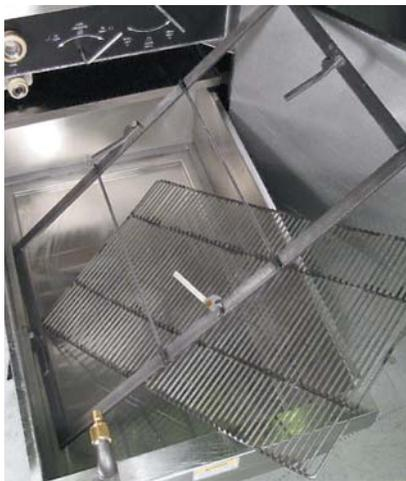
Remove the FILTER PAN and COVER.
