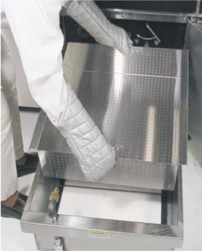
Replace the CRUMB CATCHER on the FILTER PAN.
