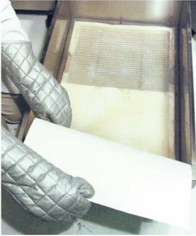
Lift the remaining piece of FILTER PAPER and place a new piece of FILTER PAPER **BELOW** the existing piece.
