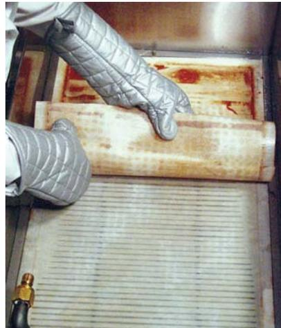
Carefully remove the top piece of **FILTER PAPER** and **DISCARD**.
