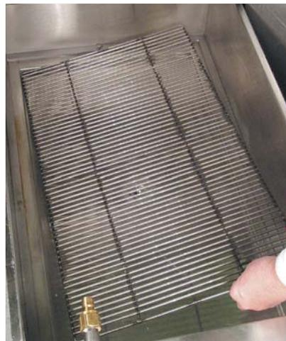
Allow the pieces to **DRY OVERNIGHT**. **BE CERTAIN NO WATER** is trapped in the FILTER PAN tubing by turning the pan upside down.
