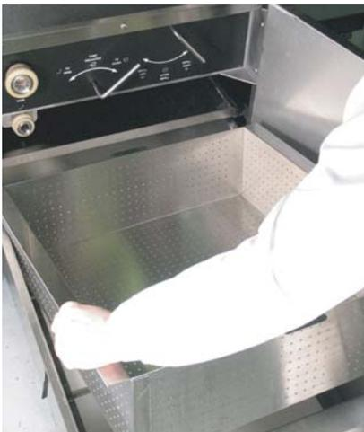
Remove and wash the **CRUMB CATCHER** using a non-soap degreaser cleaning solution. Allow the **CRUMB CATCHER** to **COMPLETELY DRY** before placing it back in the **FILTER PAN**.
