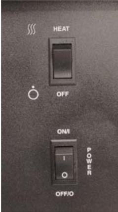
Place the POWER SWITCH in the OFF position.
