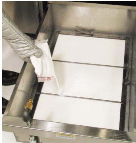
Add **1 PACKAGE** of FILTER POWDER to the FILTER PAN.
