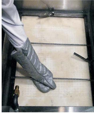
Replace the HOLD-DOWN BRACKET and **SECURELY LOCK** all 4 handles.
