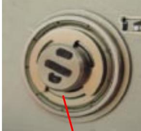
Install the drive roller with this mark at the rear.
