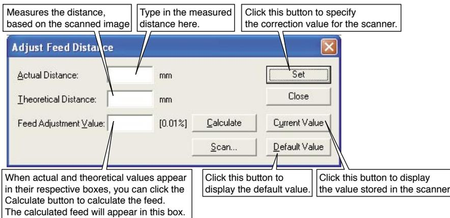
(5) Type the distance between a and c measured with a glass scale in the "Actual" box.
