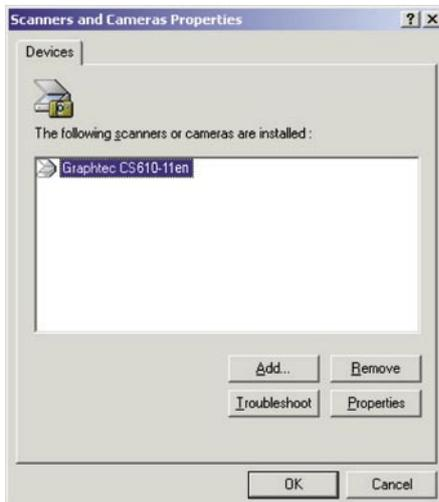
Ensure that “Graphtec CS610-11eN” is indicated here.
