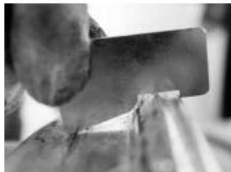
Photo 1. Acceptable Rim Flange Wear Condition
