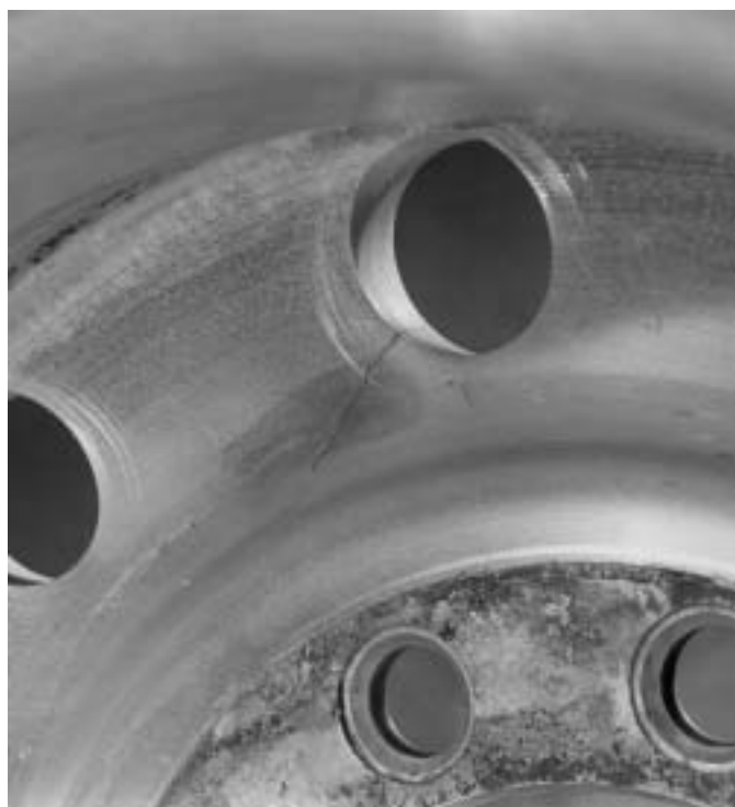
Inspect both sides of disc area for hand hole cracks. If cracks are found, remove the wheel from service.
