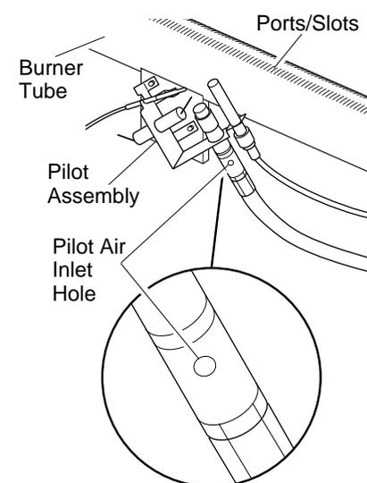
**Figure 26 - Pilot Inlet Air Hole**
