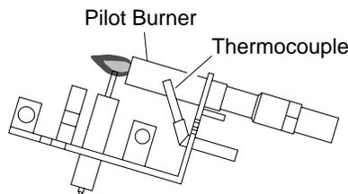
Figure 23 - Correct Pilot Flame Pattern
