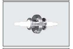
(Simultaneous operation of two systems at different pressure levels, stainless steel/FFKM, leak rate  $< 10^{-3}$  mbar x l/s for pressure differences  $\geq 500$  mbar.)
