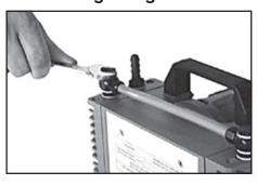
■ Use open-ended wrench to assemble screw-in fittings with connection hoses to all pump heads.
