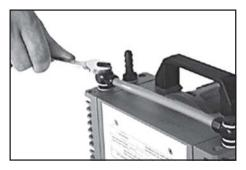
Use open-ended wrench, remove screw-in fittings from all pump heads.
