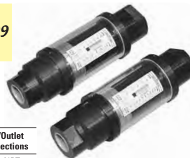
Tools needed for checking transmission cooler flow on 943, 953, 963 and 973 Track-Type Loaders (Sold Separately)
