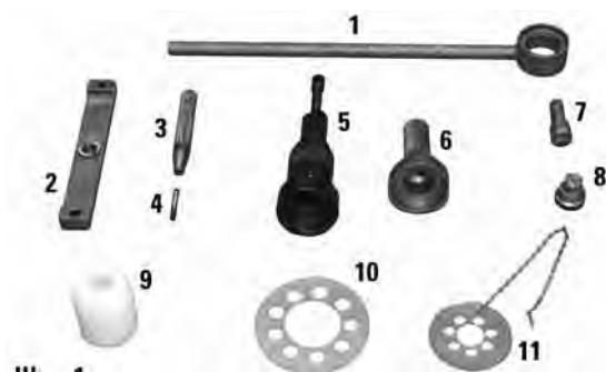
Illus. 1 Typical Excavator Hydraulic Pump and Motor Service Tools
