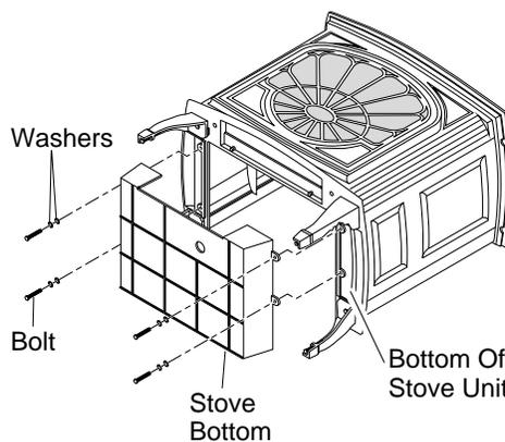
**Figure 10 - Attaching Stove Bottom (Amity™ Model Shown)**
