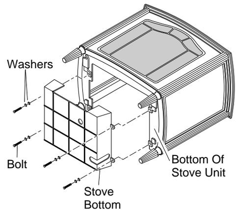
**Figure 12 - Attaching Stove Bottom (Sheraton™ Model)**
