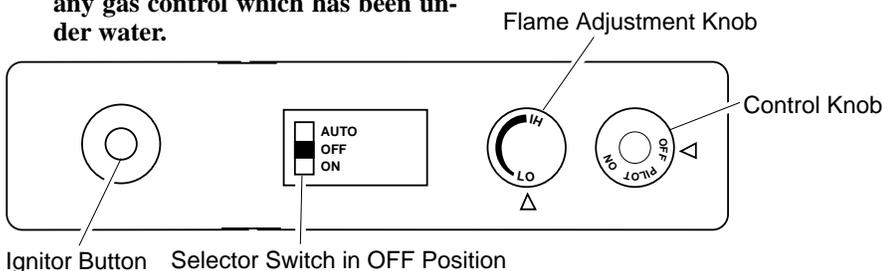
Figure 24 - Control Knob and Ignitor Button Location (Shown as Supplied, No Control Options)
