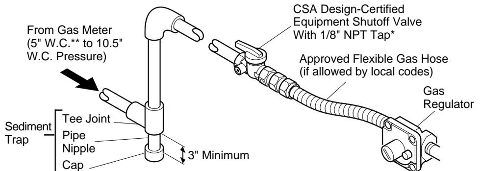
**Figure 21 - Gas Connection (SVYD18N and FSVYD18N Series)**
