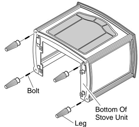
**Figure 11 - Attaching Stove Legs (Sheraton™ Model)**
