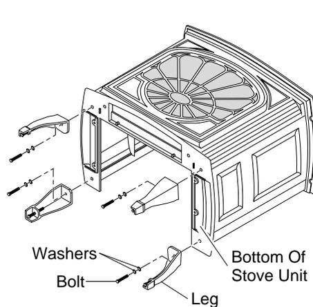
**Figure 9 - Attaching Stove Legs (Amity™ Model Shown)**
