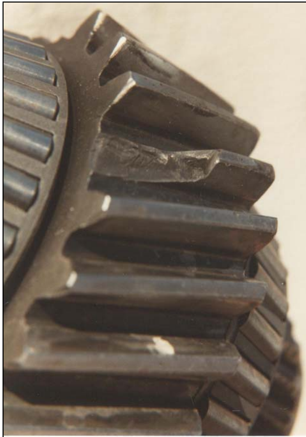
FIGURE 23. This illustrates a typical shock load tooth failure. The adjacent tooth is also cracked at the root fillet.
