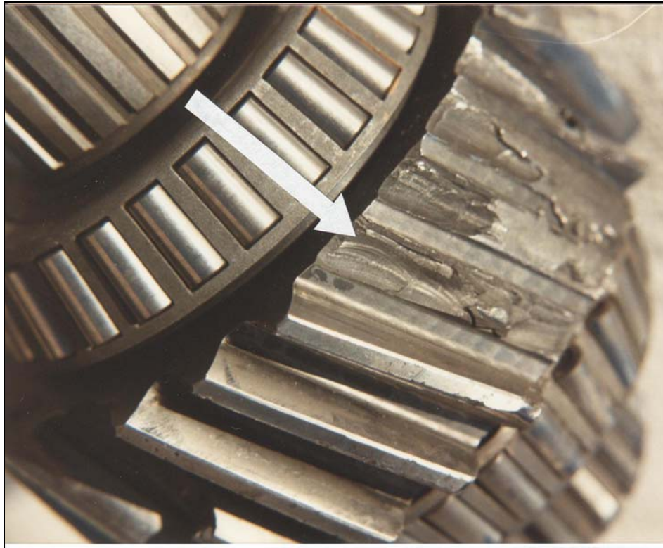
FIGURE 22. As illustrated by the arrow, this gear assembly was subjected to high load bending fatigue as evidenced by the tiny lines called “beach marks” just below the break. Beach marks are evidence of excessive tooth loads and each beach mark line corresponds to intermittent relief of the load as stress is decreased and reapplied. When a gear is loaded in this manner and subjected to repeated high load cycles, the affected teeth will fail. Stress risers in the roots such as inclusions, or deep machining marks, can initiate these failures.
