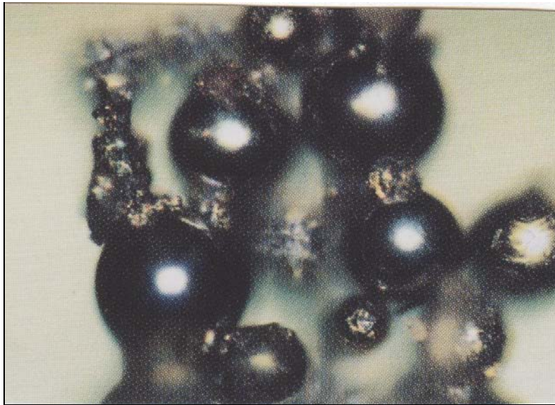
FIGURE 14. This ferrogram shows small spheres approximately 5 microns in diameter providing evidence of the onset of rolling element bearing failure. Ultrasonic testing and/or vibration analysis should be immediately carried out at bearing caps to determine if a bearing (or bearings) are showing possible failure.
