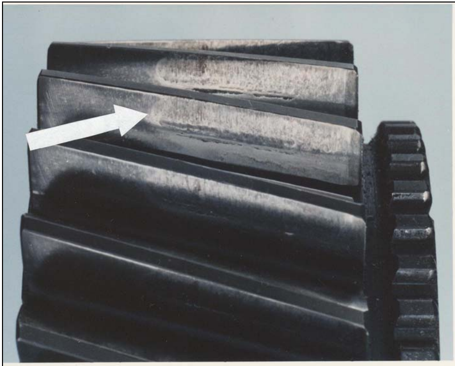
FIGURE 20. This gear shows evidence of misalignment. Note that tooth contact only covers approximately \frac{1}{3} of the teeth as indicated at the point of the arrow. The problem was located using spectroscopic oil analysis which indicated high rates of iron wear. A Ferrographic analysis confirmed higher than normal wear rates and vibration analysis confirmed the misalignment.
