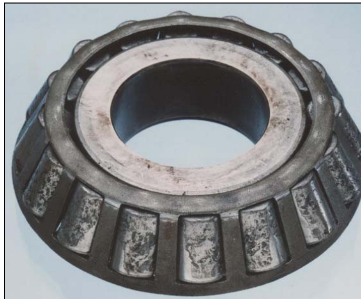
FIGURE 21. This gear drive bearing shows clear evidence of water contamination. Note the discoloration on the inner race and parts of the cage, as well as the corrosive pitting on all rolling element surfaces.
