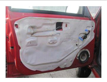
**STEP 6:** Remove the vapor barrier.
