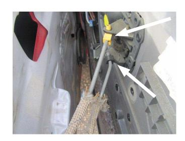
**STEP 4:** Disconnect the power door locks/power window/ power mirror wire harness connectors (if equipped).
