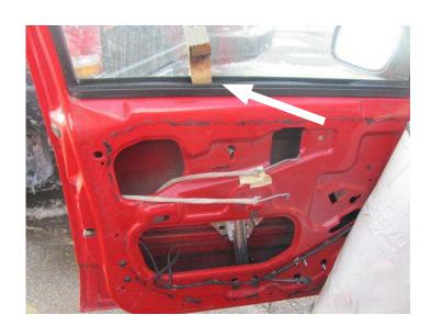
**STEP 8:** Loosen the bolts attaching the regulator to the inner door panel.
