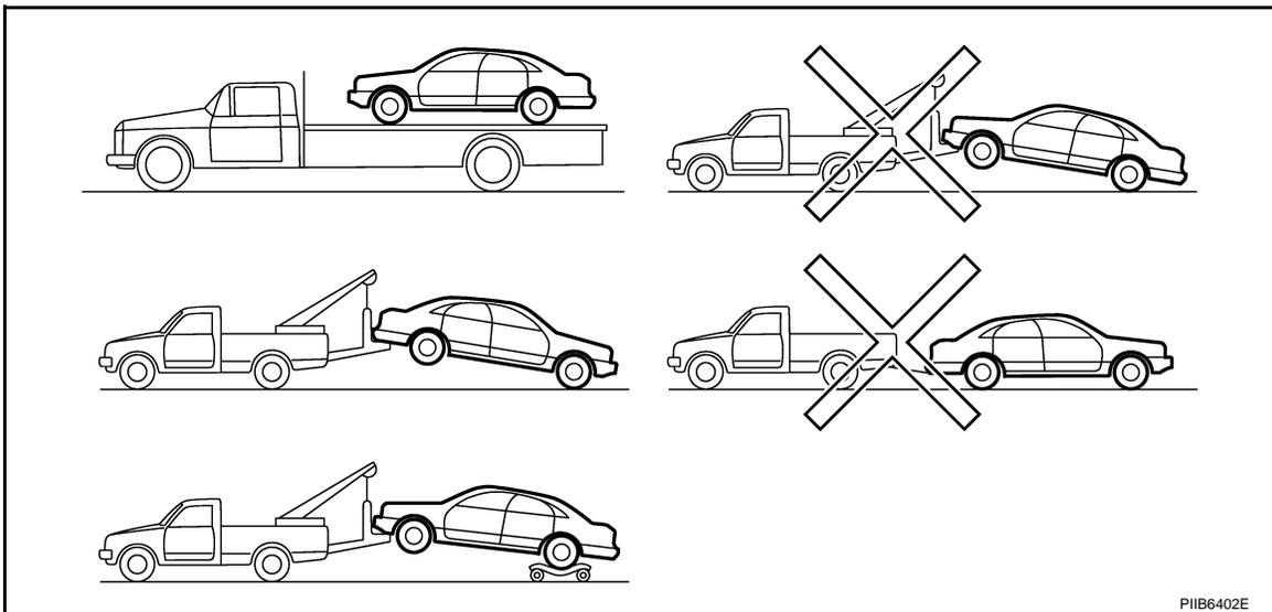
INFINITI recommends that vehicle be towed with the driving (rear) wheels off the ground or that a dolly be used as illustrated.
