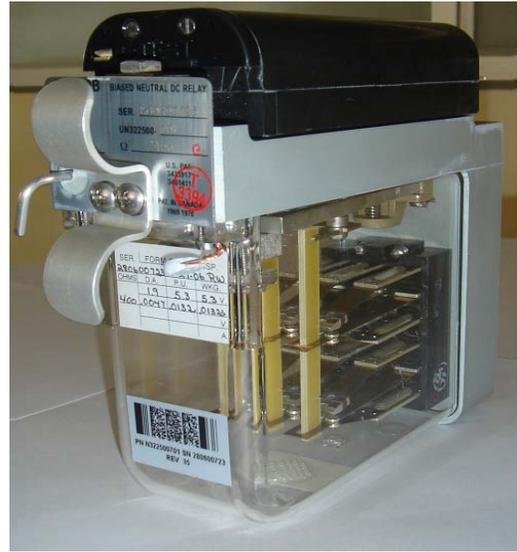
*Fig.2.7: Vital Cut-Off Relay (VCOR)*
