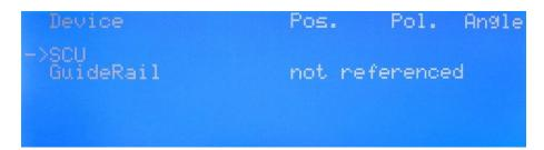
In this example the main screen shows the SCU itself and a not referenced Cable Guide Rail CGR.
