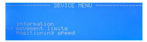
2. Navigate to "information" and press "ENTER". The device type, the serial number and the firmware version will be shown.
