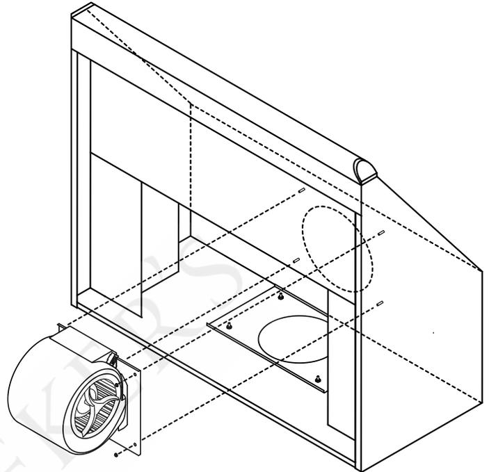
10. Remove and discard the mounting plate attached to the blower motor.
