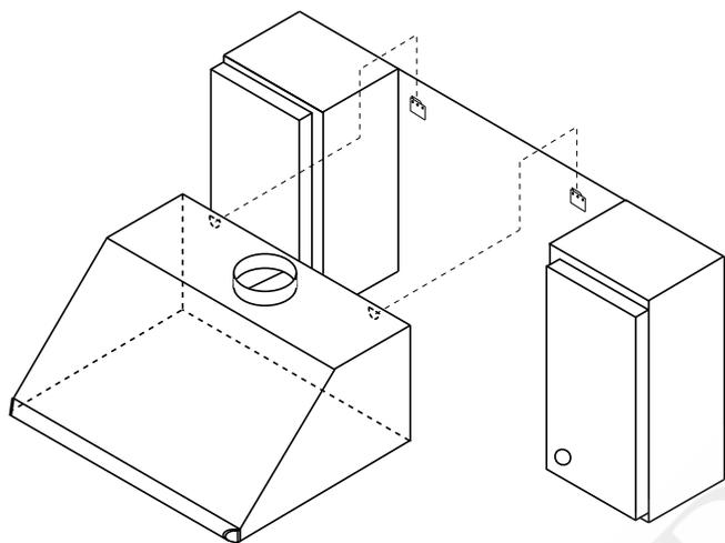
4. Lift the hood into its final position and mark the desired locations for the anchors or wood screws through the mounting slots on the back and top of the hood.
