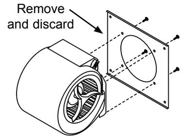
12. Attach the mounting plates removed in step 11 (rear mounting plate) to the blower motors.
