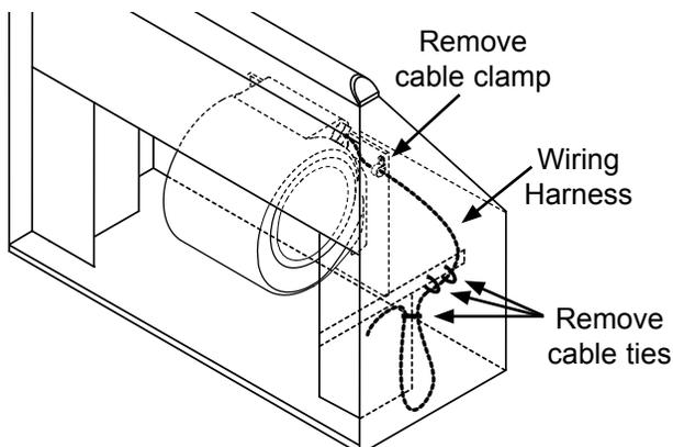
8. Disconnect the wiring harness connector from the blower motor.
