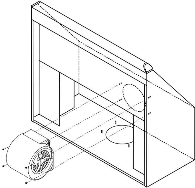
10. Insert the opening on the blower motor into the hole inside the back of the hood. The connector on the motor must be toward the bottom of the hood. Attach it using four (4) nuts.
