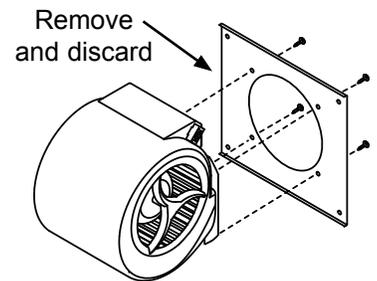
11. Remove the four (4) nuts that hold the rear mounting plate in place and remove it. See below.
