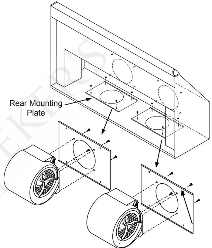
13. Insert the opening of each blower motor assembly into the holes inside the back of the hood. The connector on the motors must be toward the bottom of the hood. Attach them with four (4) nuts each.
