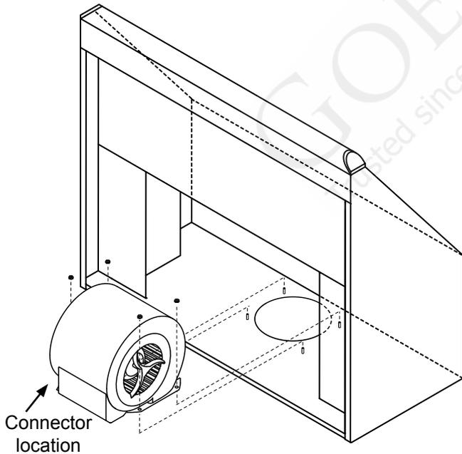
11. Route the wiring harness as shown. Secure the harness to the motor assembly with the cable clamps supplied with the hood in the positions shown below.
