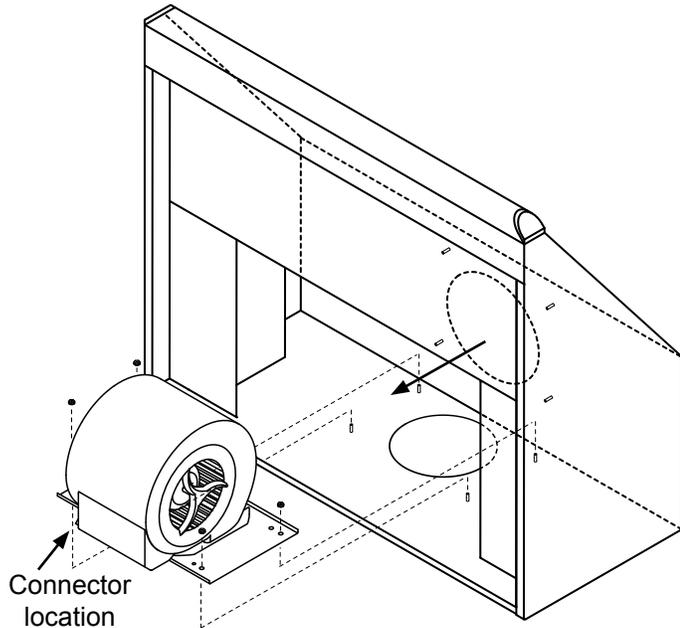
14. Route the wiring harness as shown. Secure the harness to the motor assembly with the cable clamps supplied with the hood in the positions shown below.
