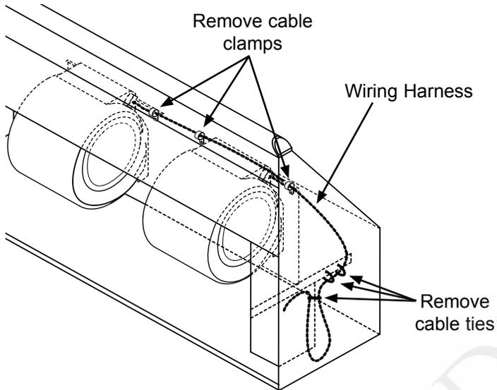
8. Disconnect both wiring harness connectors from the blower motors.
