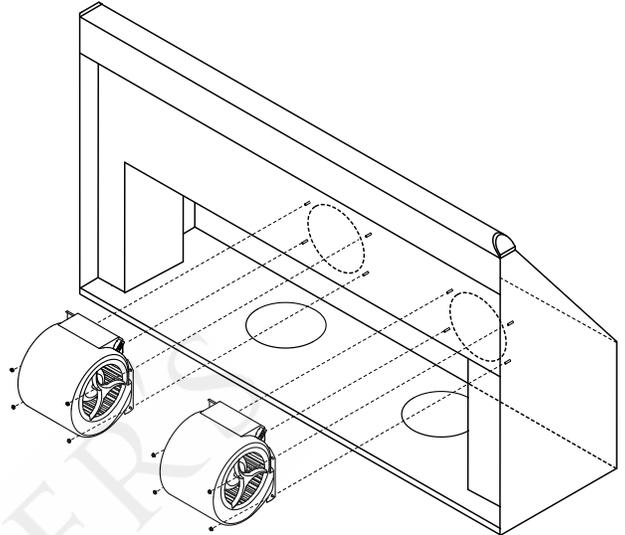
10. Insert the opening of each blower motor into the holes inside the back of the hood. The connector on the motors must be toward the bottom of the hood. Attach them with four (4) nuts each.
