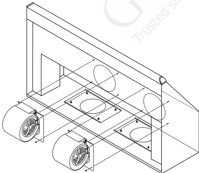
10. Remove and discard the mounting plates attached to both blower motors.
