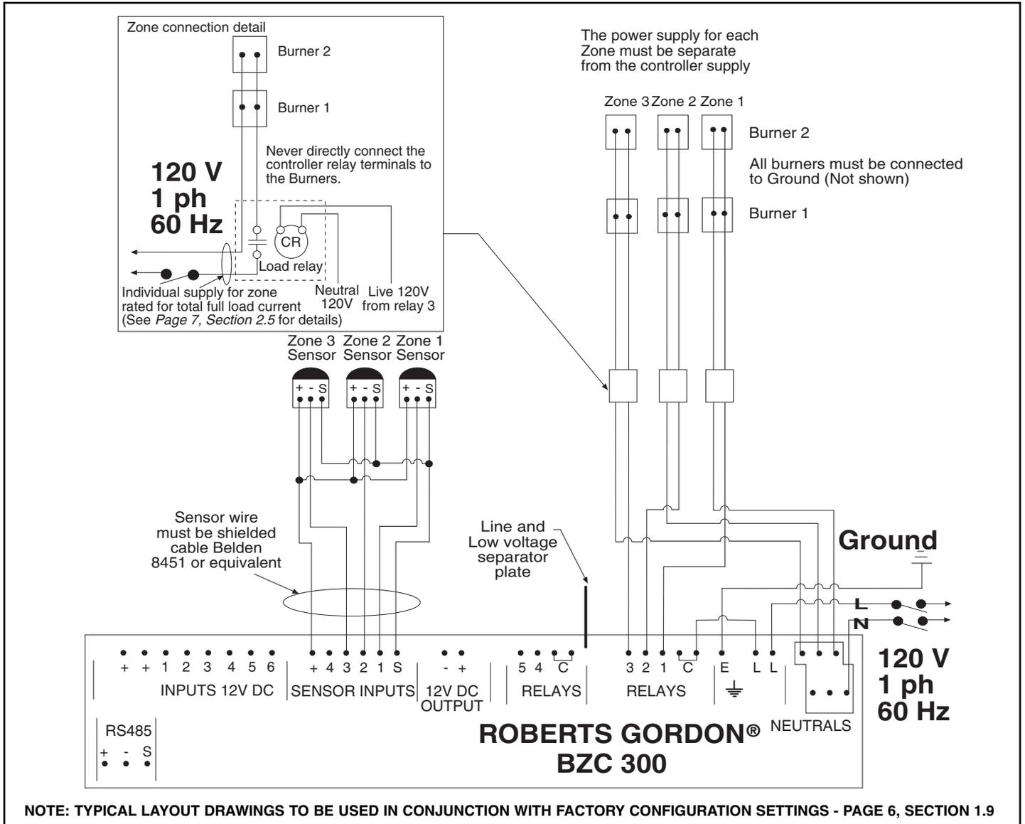
FIGURE 14 - Typical VANTAGE® II and VANTAGE® HE Unitary External Wiring Diagram
