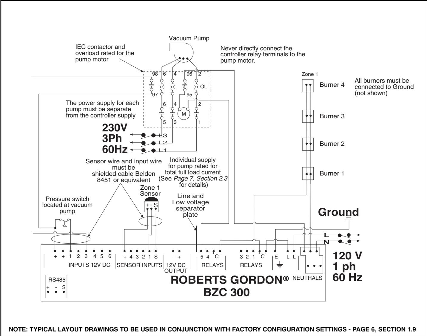
FIGURE 26 - Typical 3ph Pump Trip Indication External Wiring Diagram
