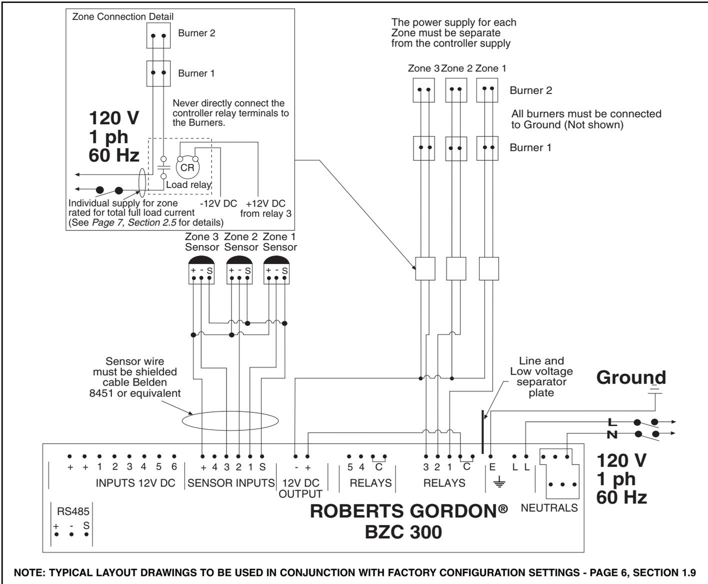
FIGURE 15 - Alternate Unitary External Wiring Diagram (12V DC switching)
