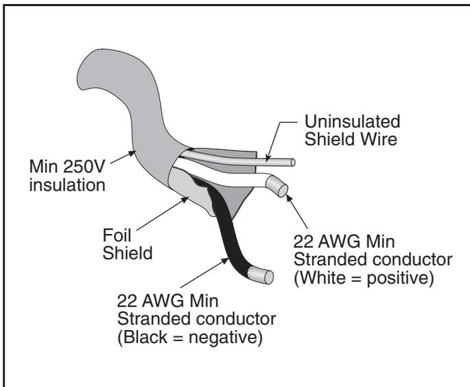
**FIGURE 10 - Shielded Cable Detail****3.3.6. Sensor Mounting**
