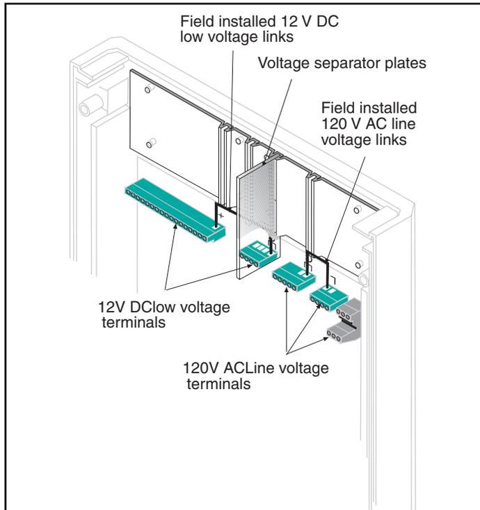
**FIGURE 9 - Separator Plate Removal Detail**
