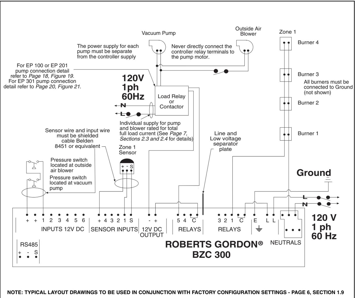
FIGURE 25 - Typical 1ph Pump with Outside Air Blower External Wiring Diagram (12V DC Switching)
