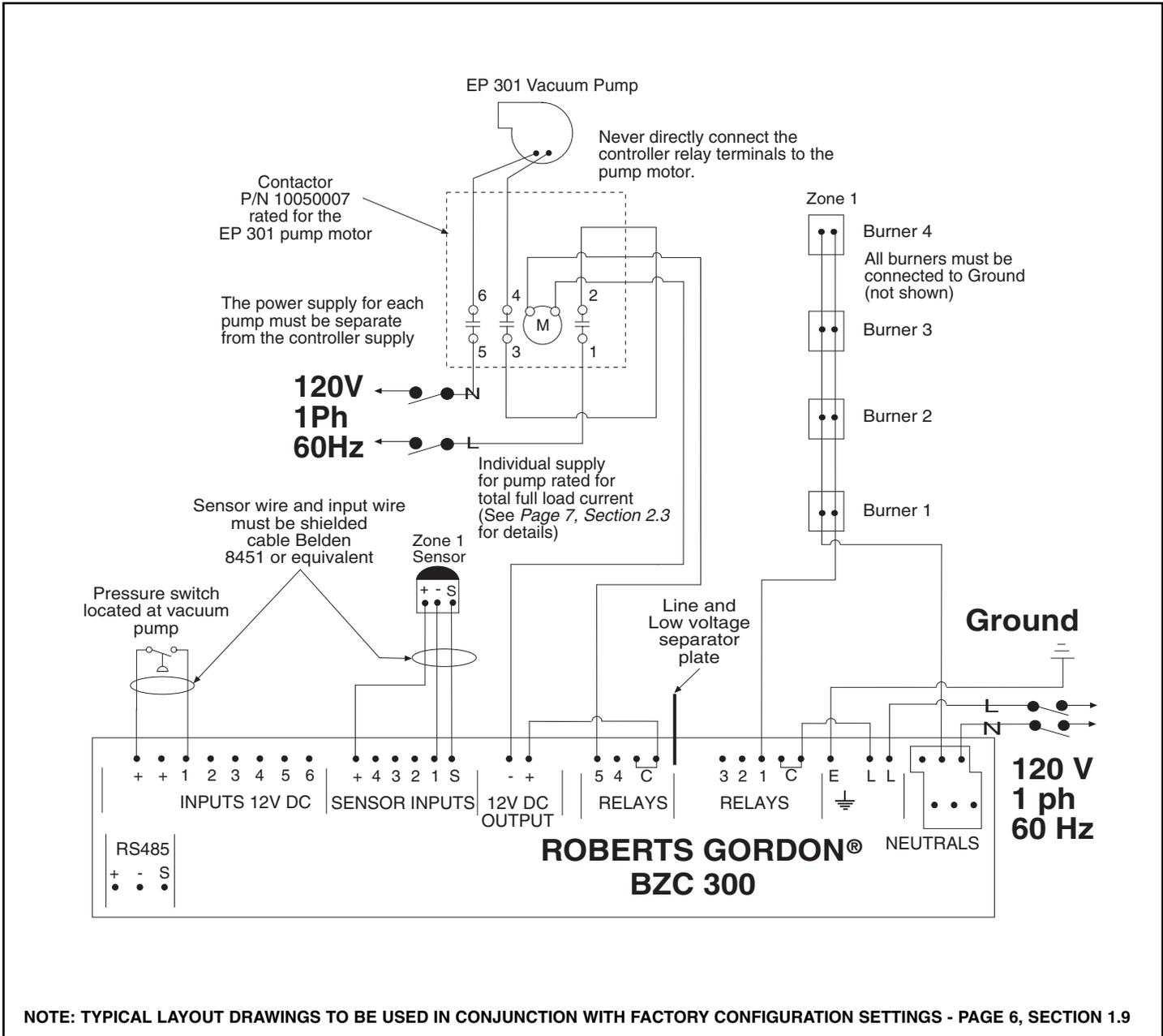
FIGURE 21 - Typical EP 301 Pump Contactor External Wiring Diagram (12V DC switching)
