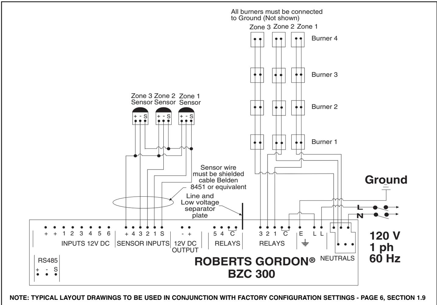
FIGURE 13 - Typical GORDONRAY® BH, CARIBE® and VANTAGE® TF Unitary External Wiring Diagram
