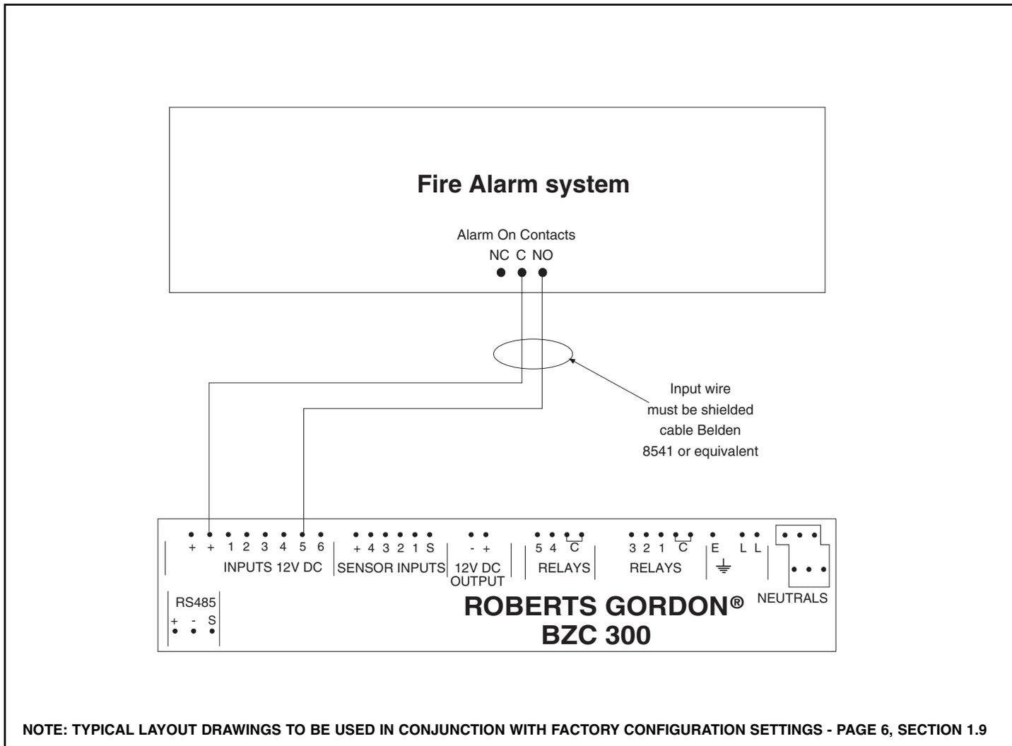
**FIGURE 30 - Fire Safety Shut Off External Wiring Diagram**
