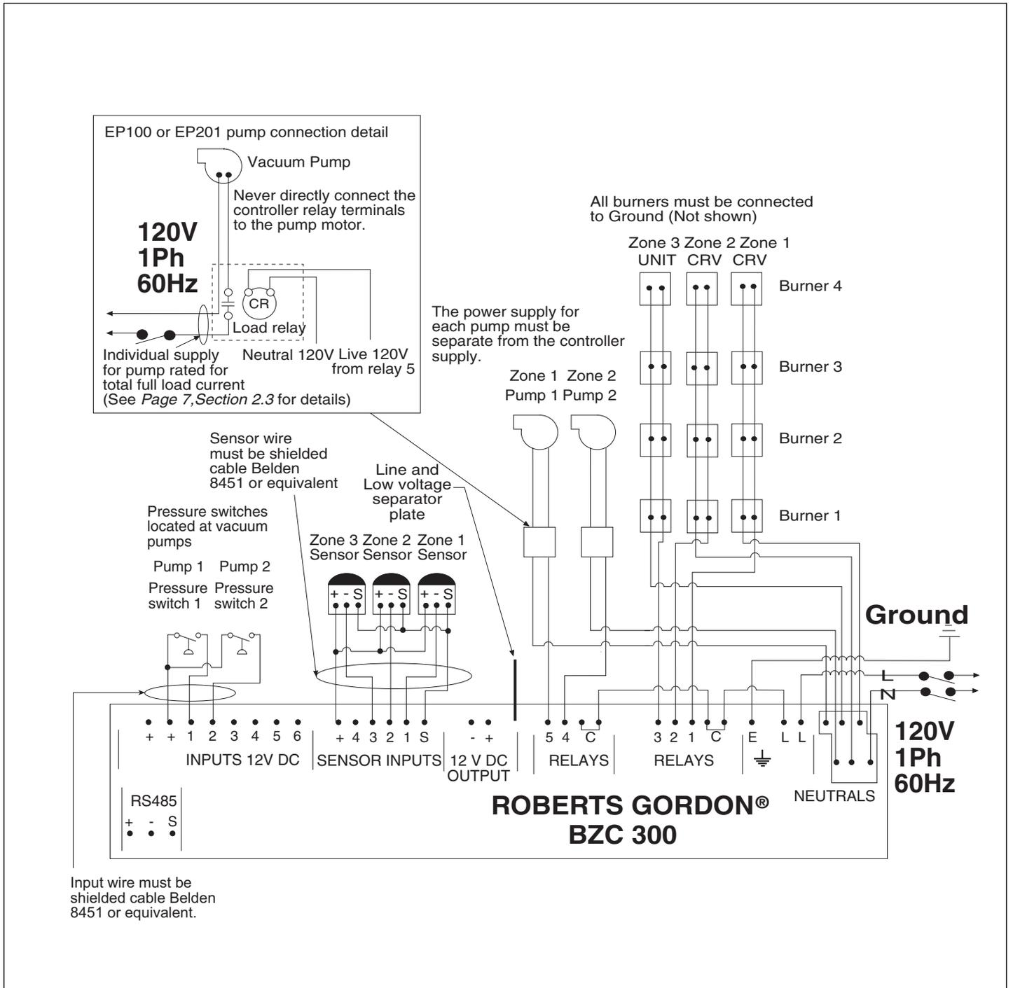
**FIGURE 4 - Example External Wiring Diagram**
