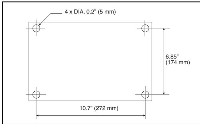
FIGURE 7 - Mounting Hole Layout
