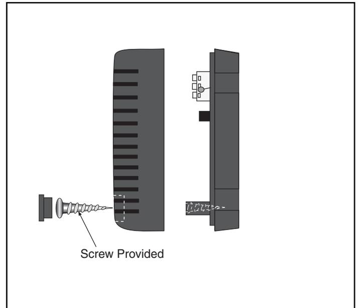
**FIGURE 11 - Sensor Cover Assembly**
