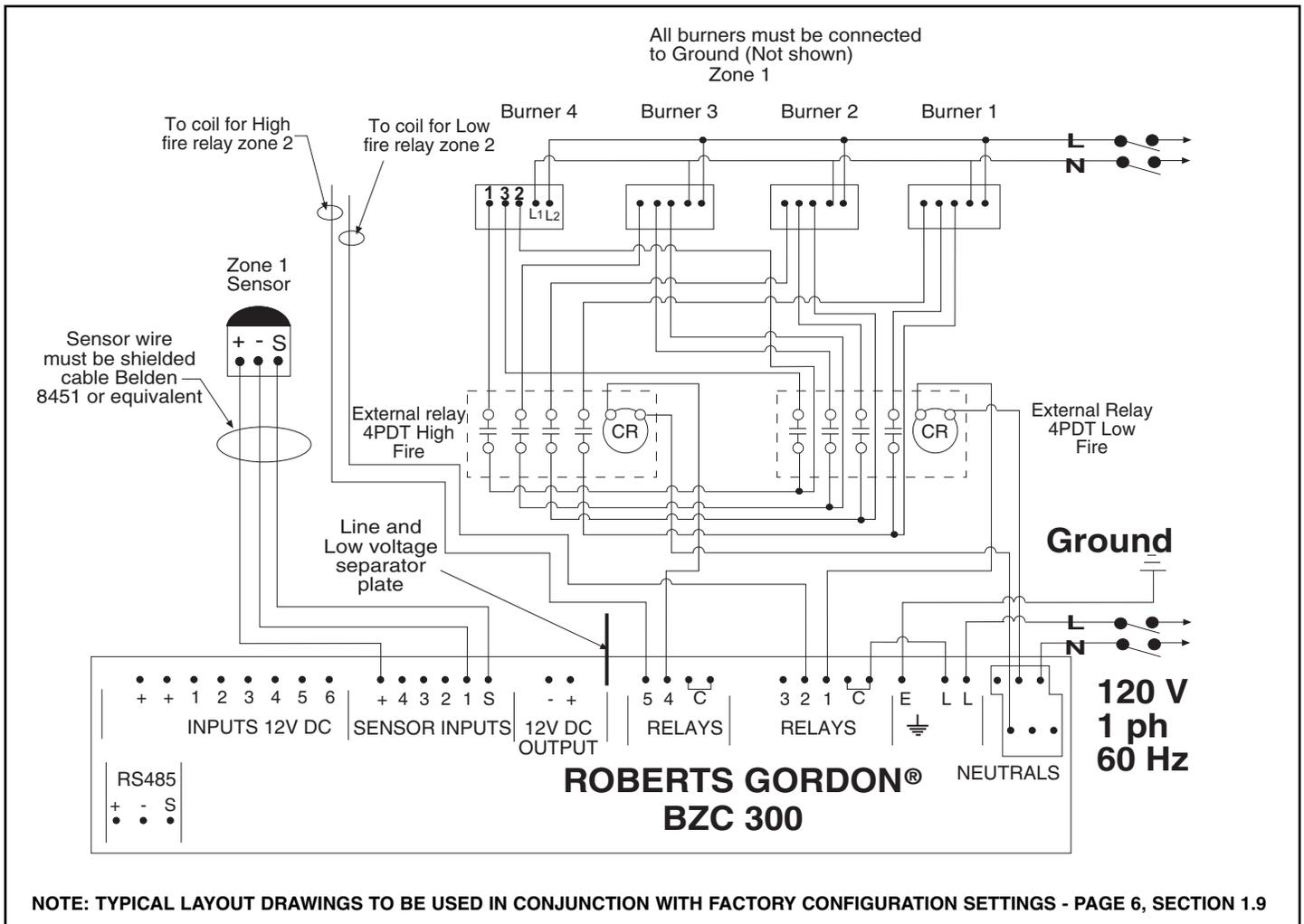
FIGURE 16 - Typical GORDONRAY® DF External Wiring Diagram
