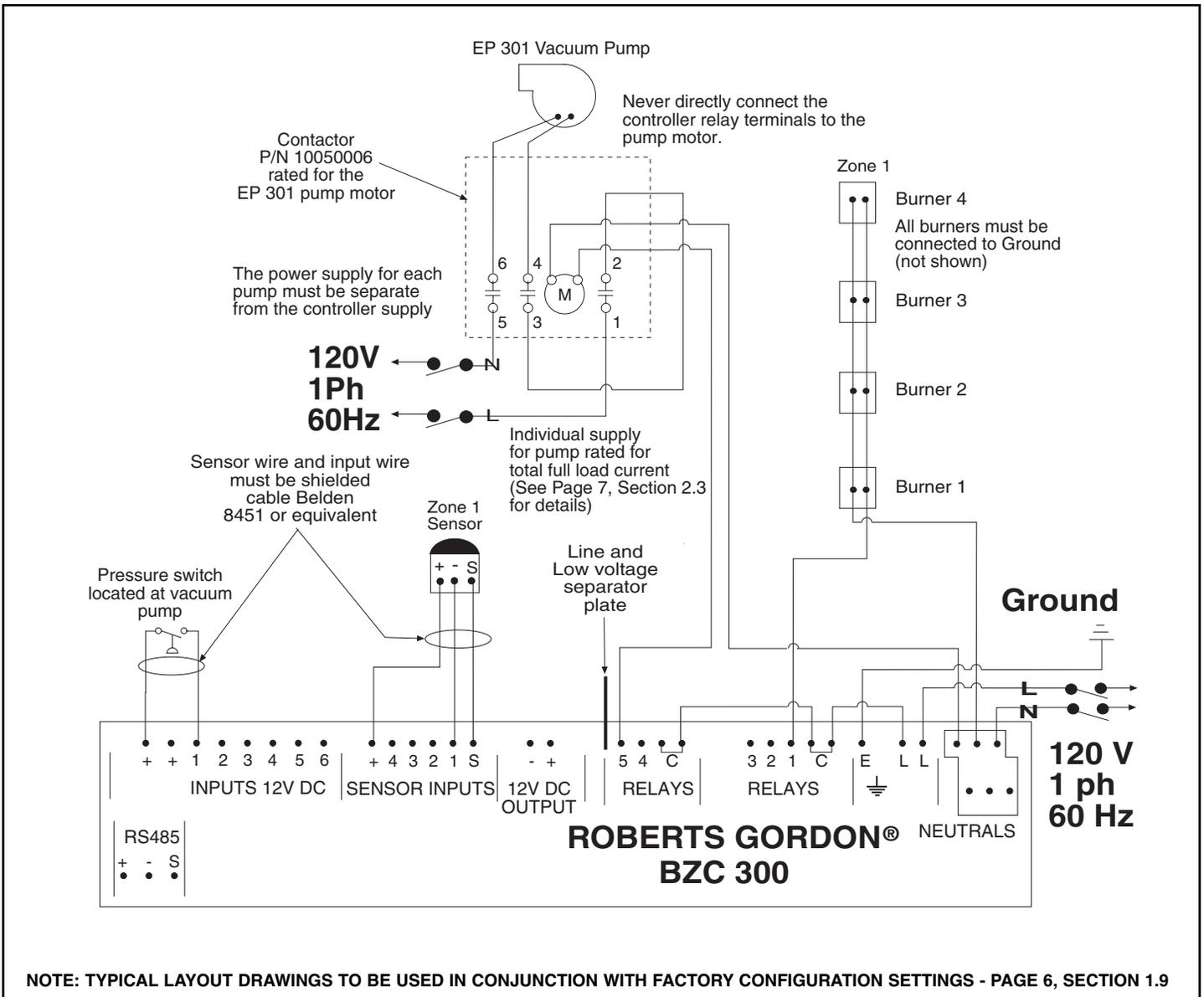
FIGURE 20 - Typical EP 301 Pump Contactor External Wiring Diagram
