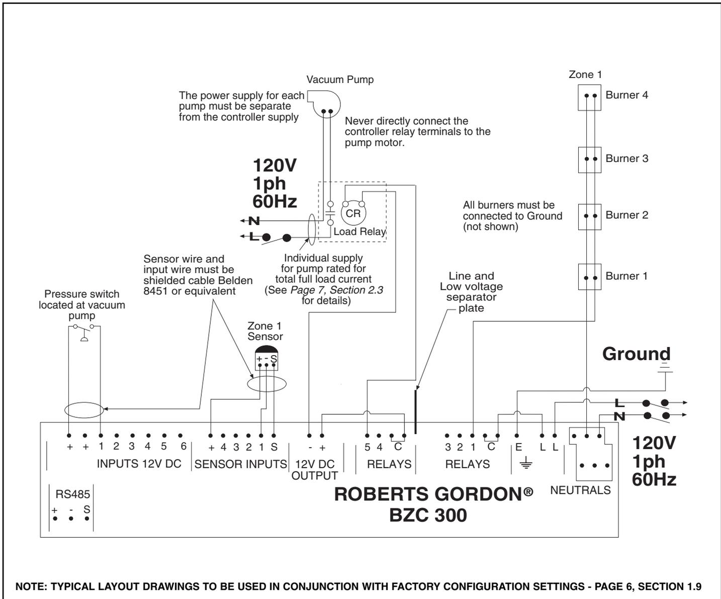
FIGURE 19 - Typical EP 100 and EP 201 1ph External Wiring Diagram (12V DC switching)
