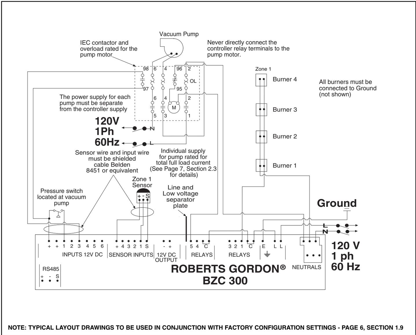
FIGURE 27 - Typical 1ph Pump Trip Indication External Wiring Diagram
