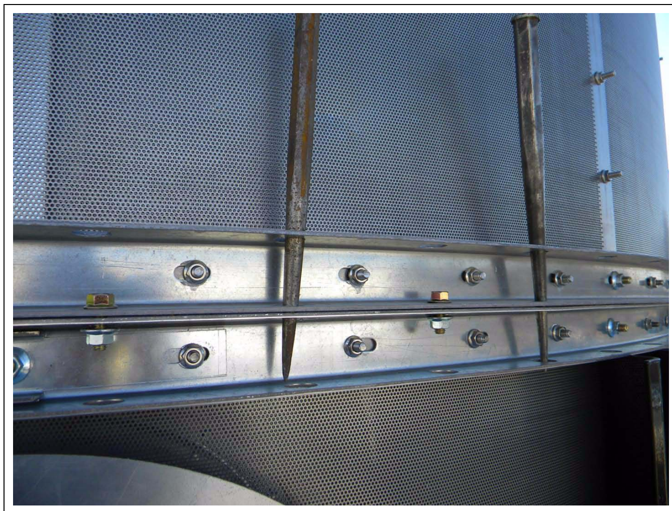
Figure 5C Line Up Punch Inserted Through Connecting Channels of Dryer
