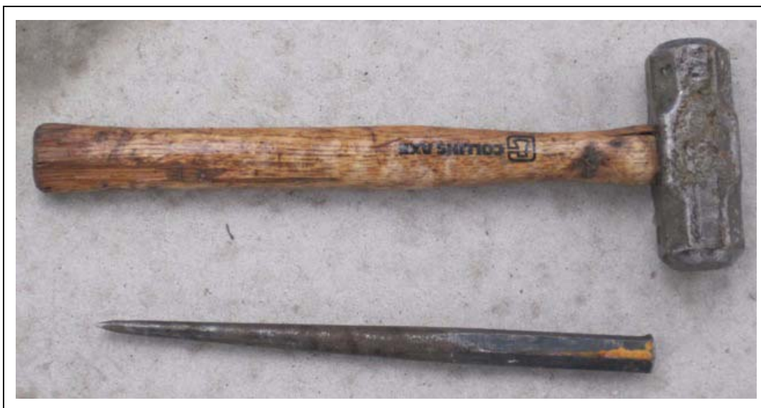
Figure 5B Line Up Punch and Hammer
