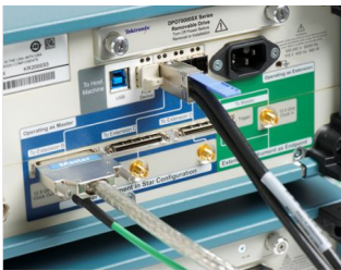
UltraSync connection on instrument with Master role
