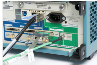
UltraSync connection on instrument with Extension role
