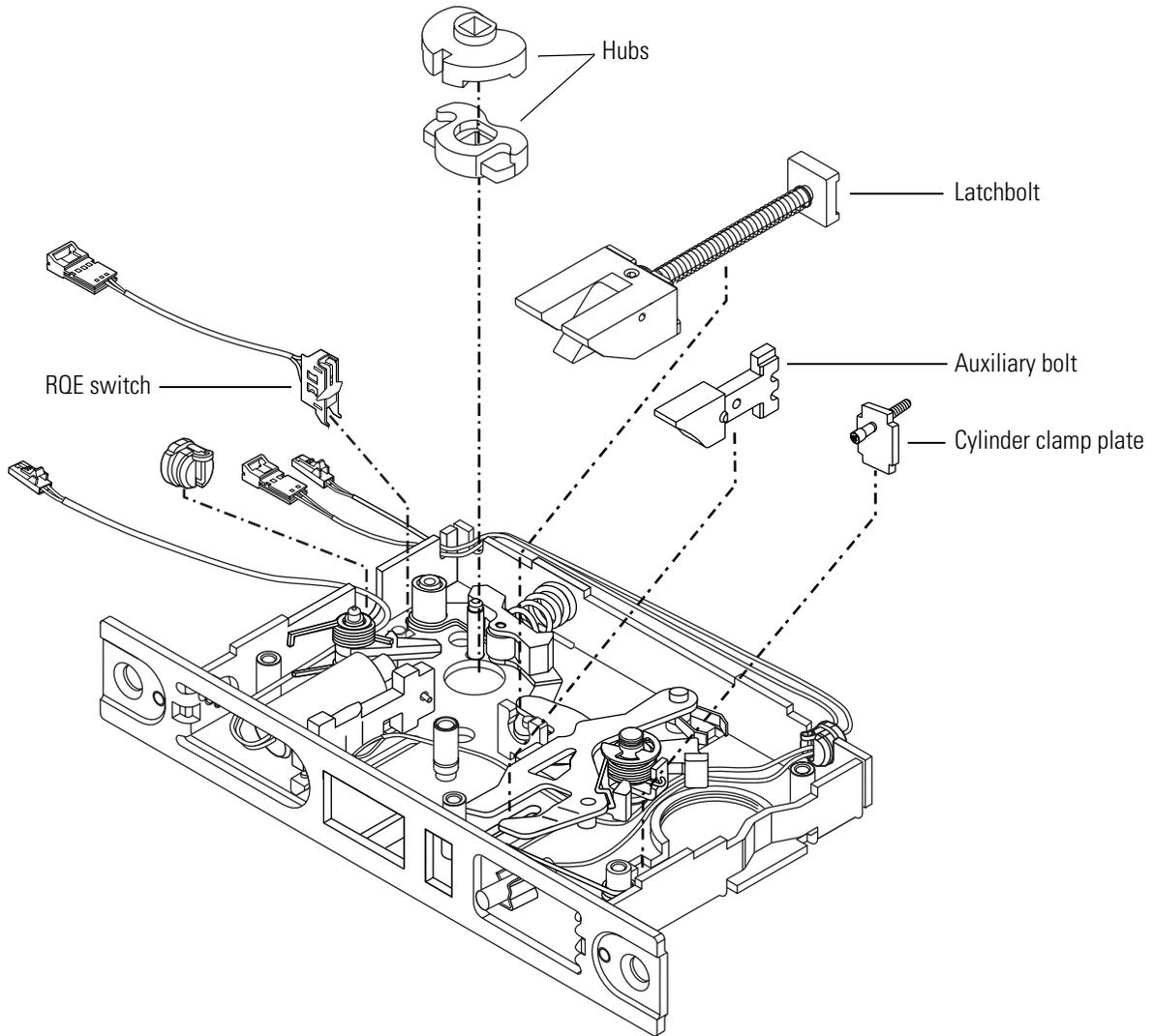
**Figure 3.27** Overview of changing the hand and bevel (LHRB orientation shown)
