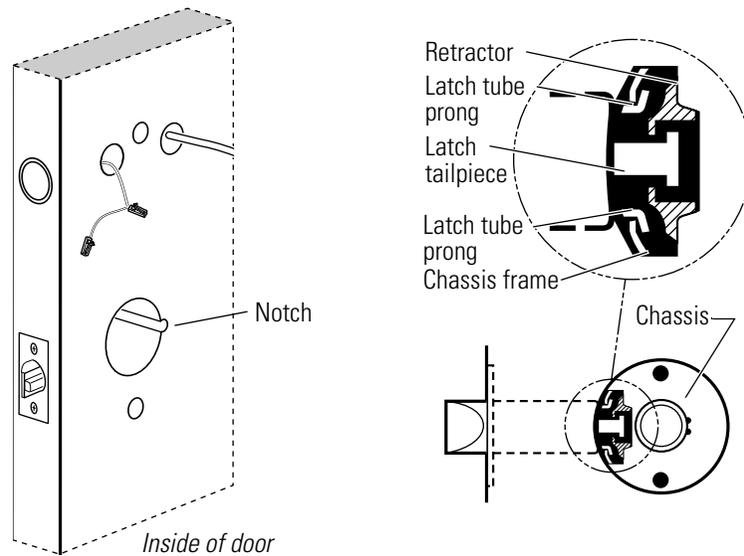
**Figure 4.12** Reinstalling the lock chassis and engaging the retractor in the latch
