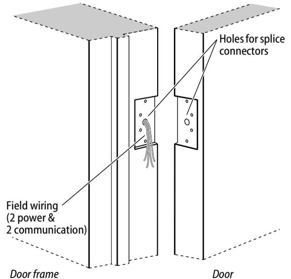
Figure 6 Preparing for the wire transfer hinge
