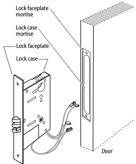
Figure 3 Mortising for the lock case and faceplate
