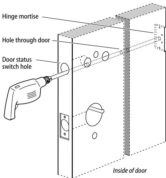
Figure 3 Drilling the hole for the field wire harness
