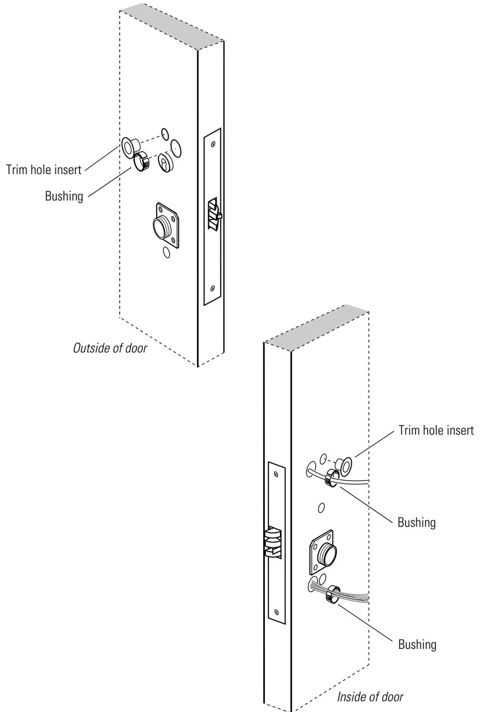
**Figure 3.8** Removing the trim hole inserts and bushings from the door
