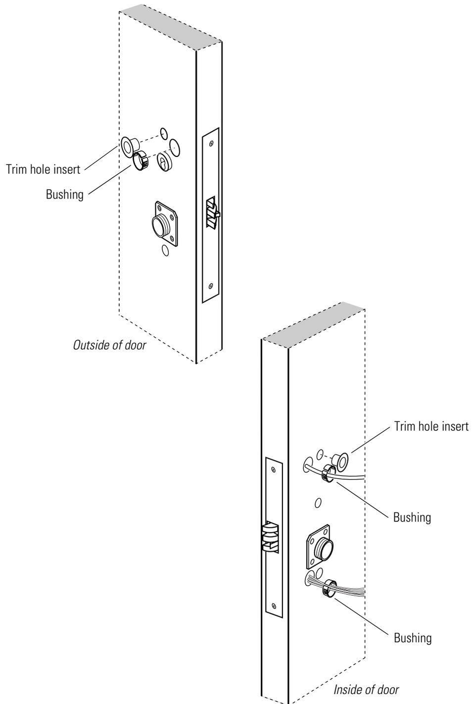
**Figure 3.18** Reinstalling bushings and trim hole inserts
