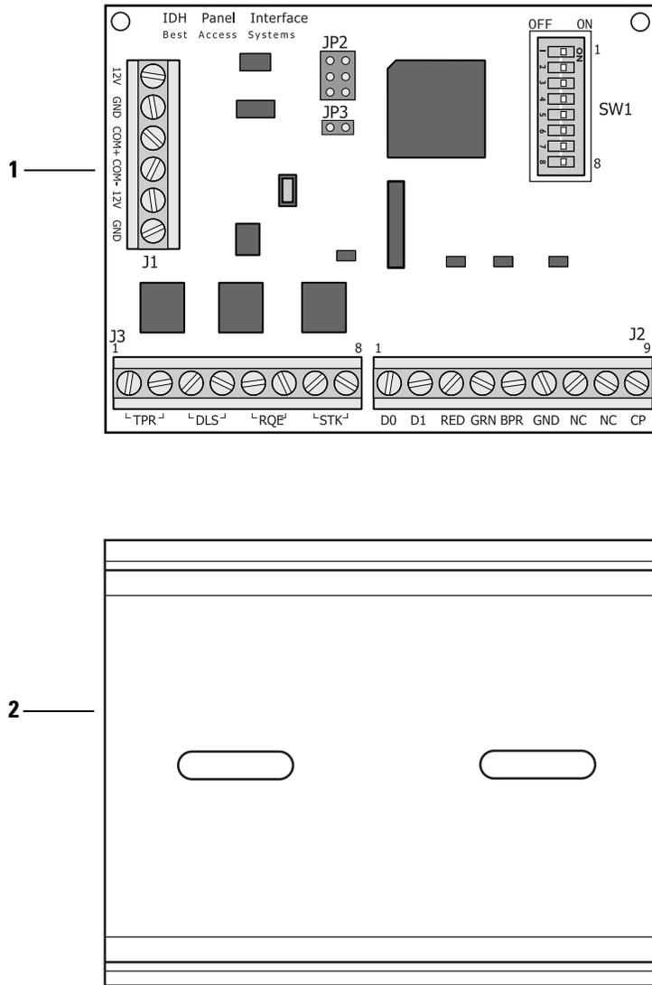
**Figure 2.11** Panel interface module components
