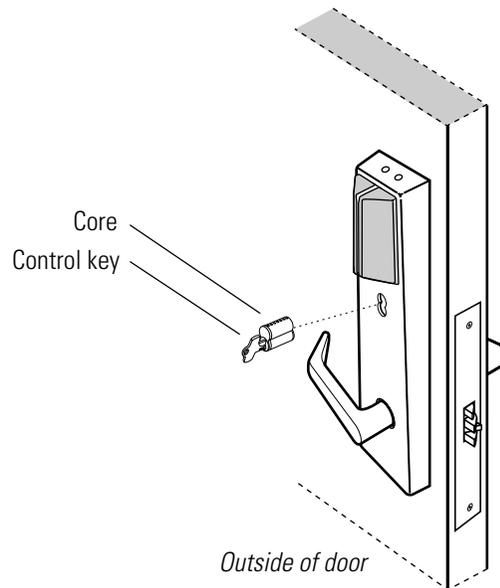
**Figure 3.1** Removing the core
