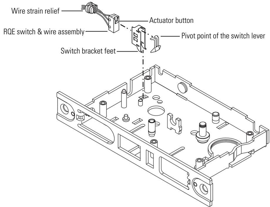
**Figure 3.29** RQE switch assembly anatomy (LH orientation of RQE shown)
