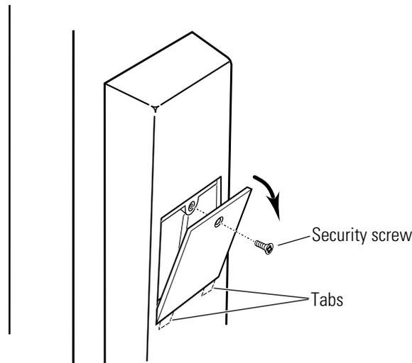
**Figure 4.4** Removing the access door
