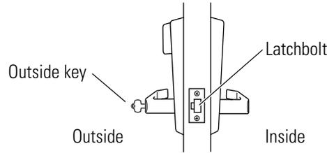
**Figure 2.2** Understanding cylindrical function drawings
