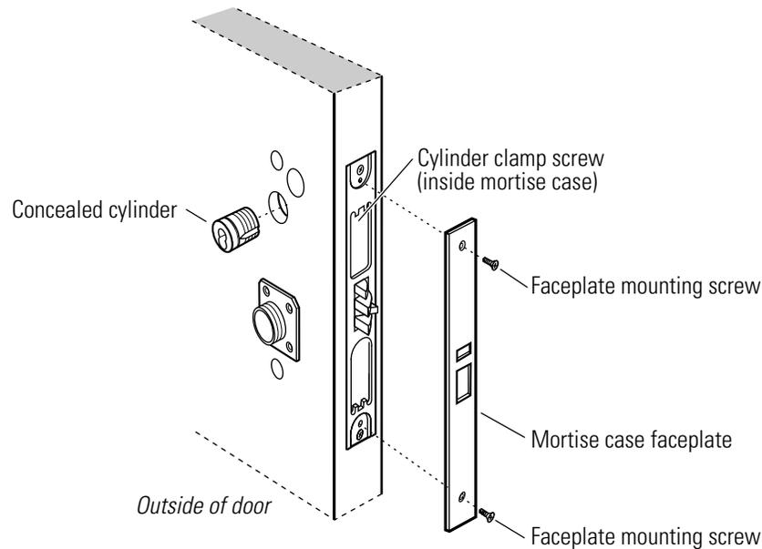
**Figure 3.17** Reinstalling the cylinder and mortise case faceplate
