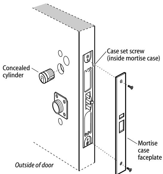
Figure 11 Installing the cylinder and mortise case faceplate
