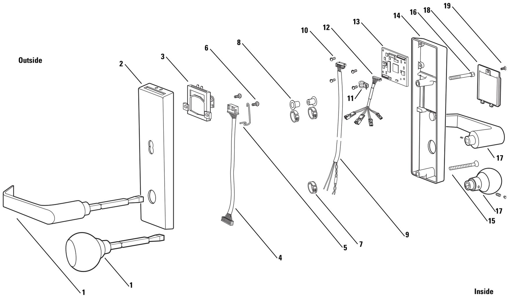
**Figure 2.5** Magnetic stripe insertion card reader and trim exploded diagram
