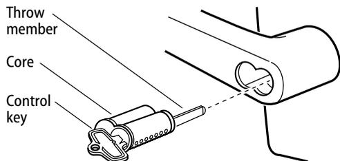
Figure 18b Installing the core
