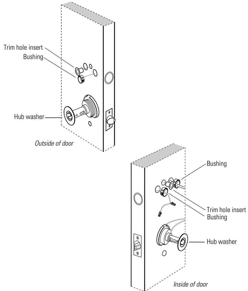
**Figure 4.7** Removing the bushings, trim hole inserts, and hub washers
