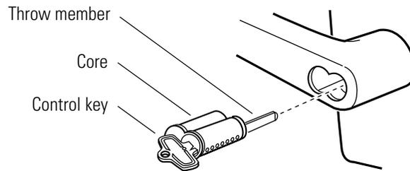
**Figure 4.20** Reinstalling the core and throw member (lever shown)
