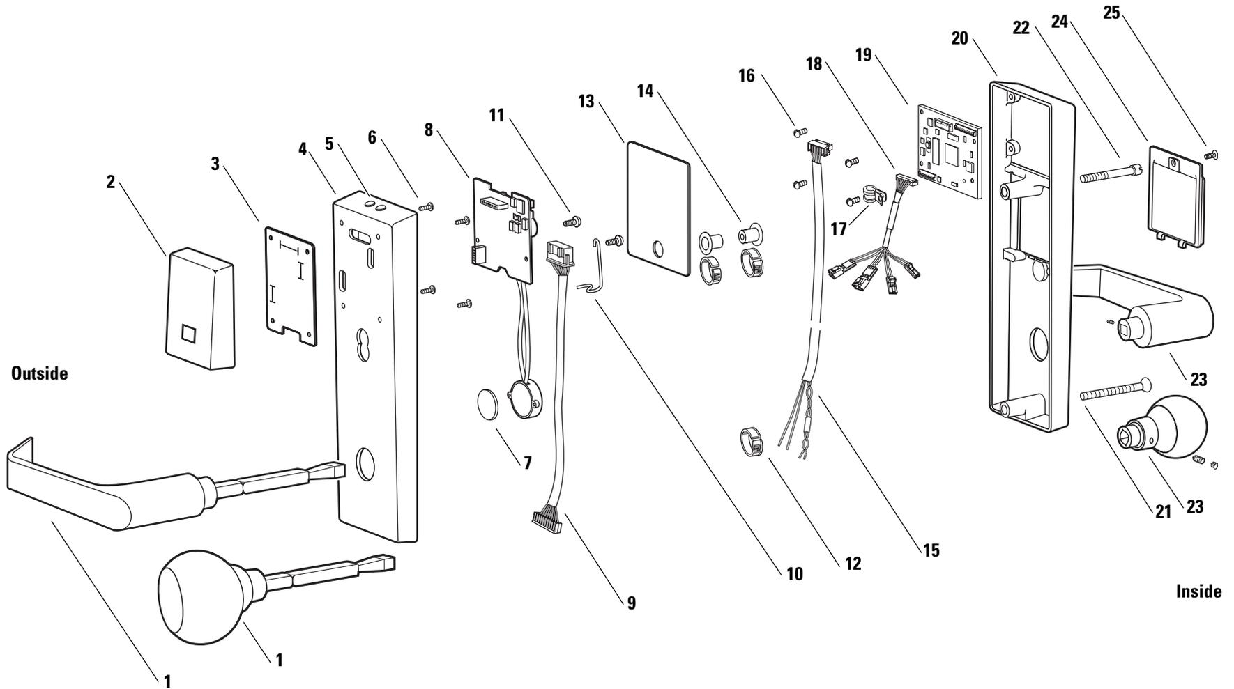
Figure 2.3 Proximity card reader and trim exploded diagram
