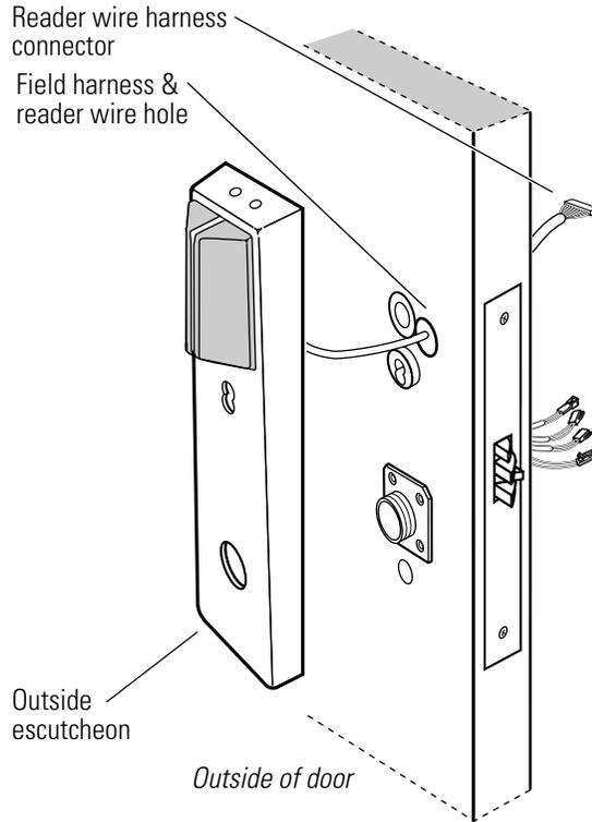
**Figure 3.7** Removing the outside escutcheon from the door
