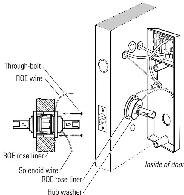
**Figure 4.22** Removing and reinstalling the RQE rose liner
