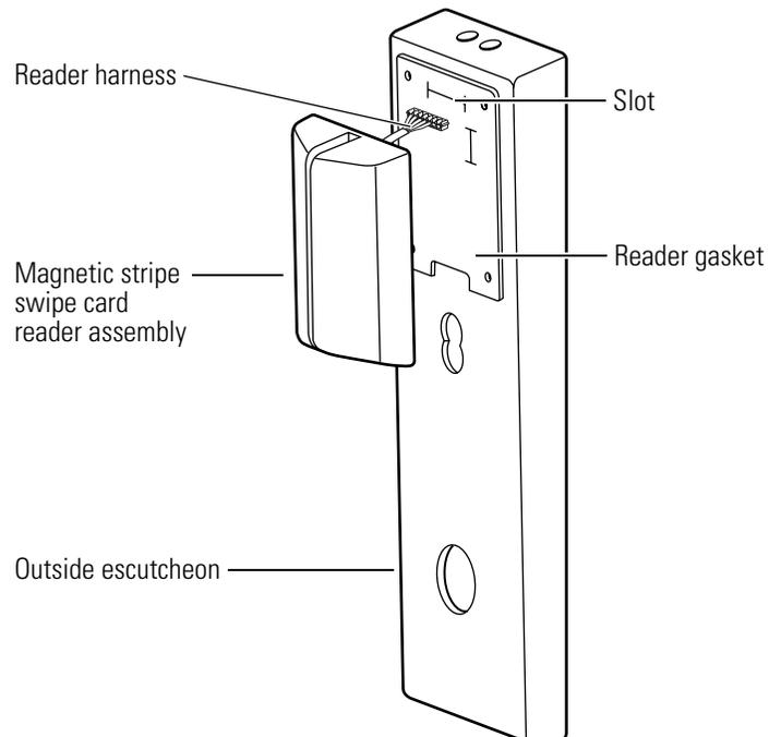
**Figure 5.5** Removing and reinstalling the magnetic stripe swipe card reader
