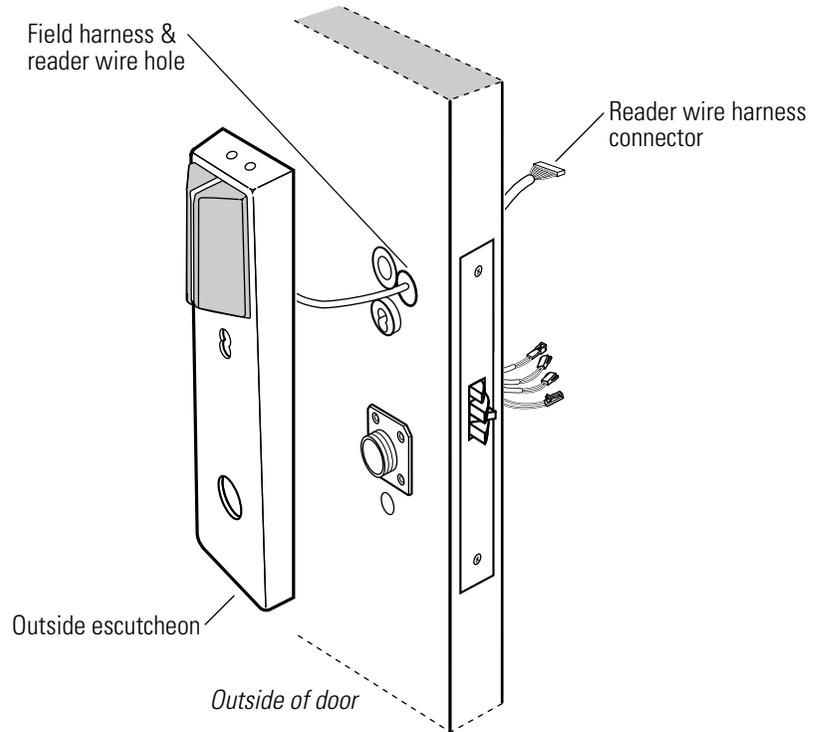
**Figure 3.19** Feeding the reader wire harness connector through the door
