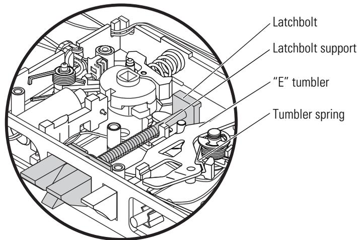
**Figure 3.42** Positioning the tumbler spring
