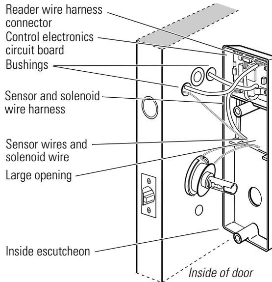
**Figure 4.16** Connecting the reader wire harness to the control electronics circuit board
