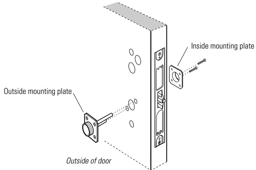
**Figure 3.16** Reinstalling the mounting plates
