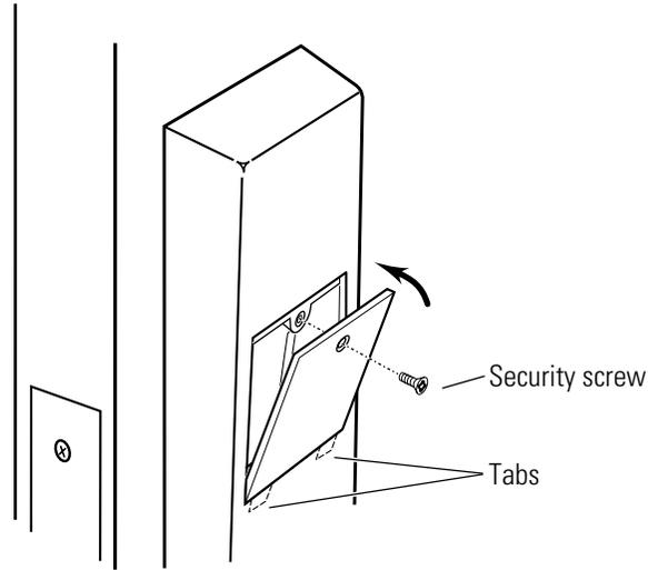
**Figure 3.25** Reinstalling the access door
