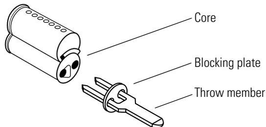
**Figure 4.19** Reinstalling the blocking plate and throw member
