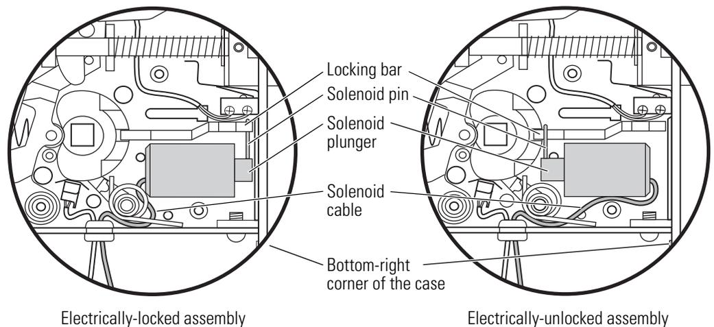
**Figure 3.36** Reversing the solenoid
