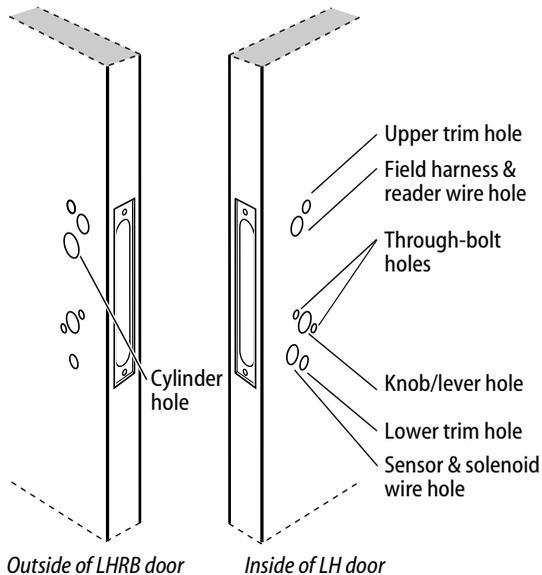
Figure 4b Drilling the LH and LHRB holes
