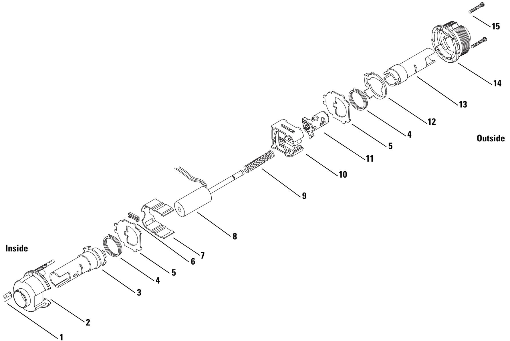
**Figure 2.9** Cylindrical chassis exploded diagram (9K DDEU function shown)
