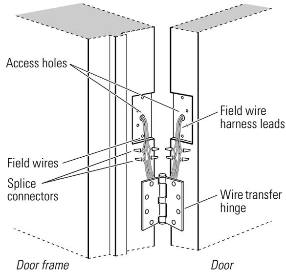
**Figure 3.12** Disconnecting the field wire harness
