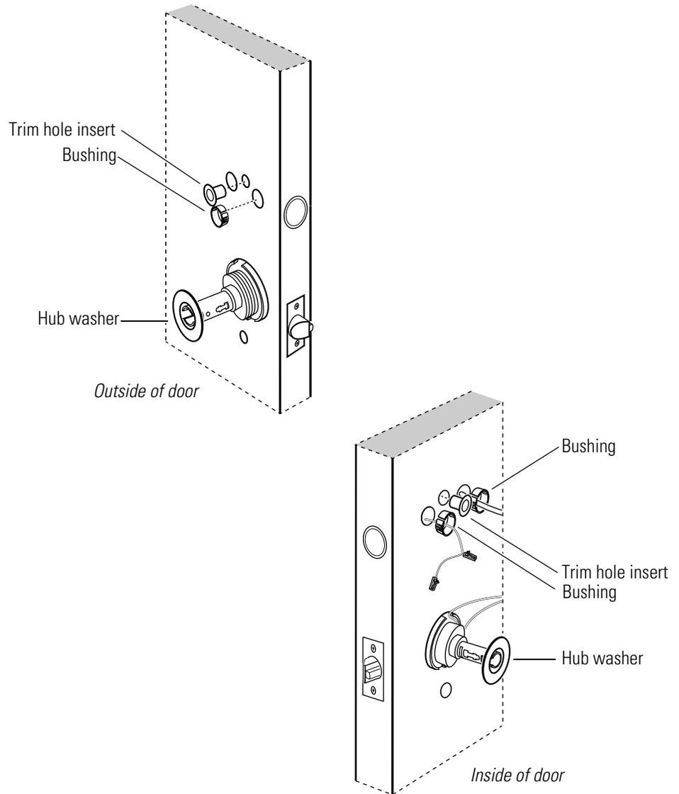
**Figure 4.14** Reinstalling trim hole inserts, bushings, and hub washers
