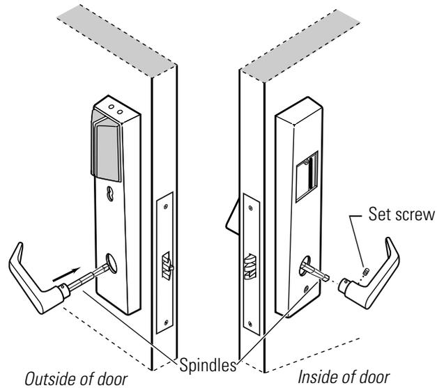
**Figure 3.23** Reinstalling the levers
