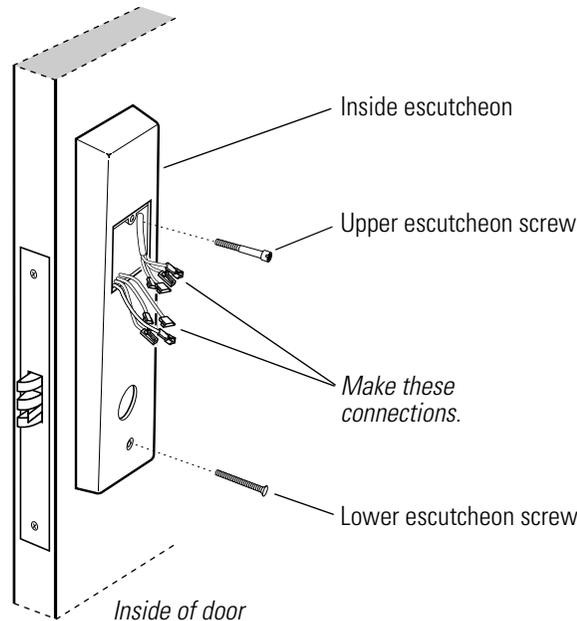
**Figure 3.21** Securing the escutcheon and completing the connections
