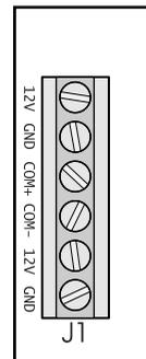
Figure 23c Connecting to the power supply
