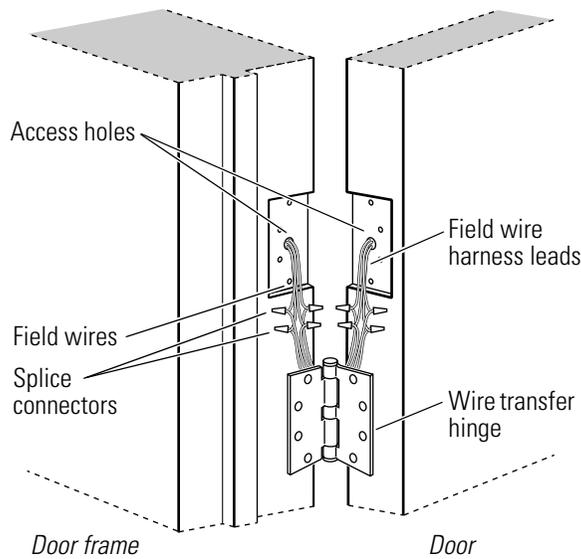
**Figure 3.14** Reinstalling the wire transfer hinge
