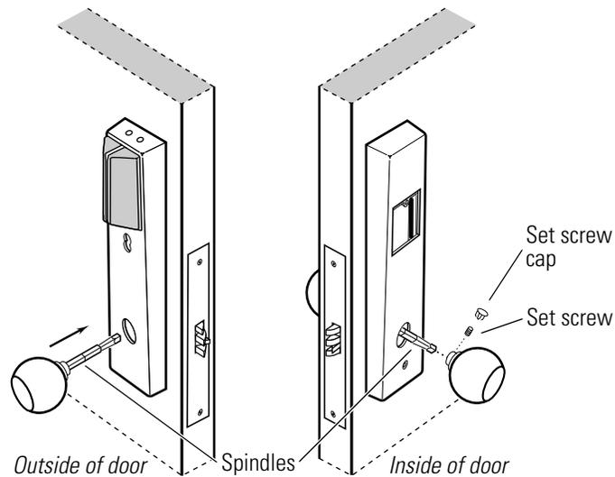
**Figure 3.22** Reinstalling the knobs
