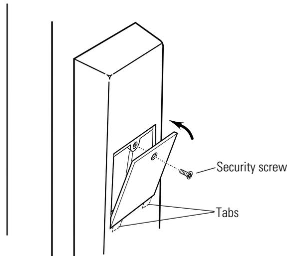
**Figure 4.21** Reinstalling the access door
