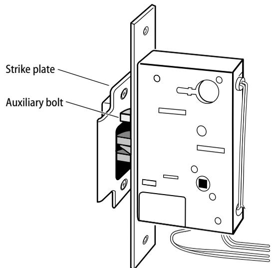
Figure 19b Positioning the strike
