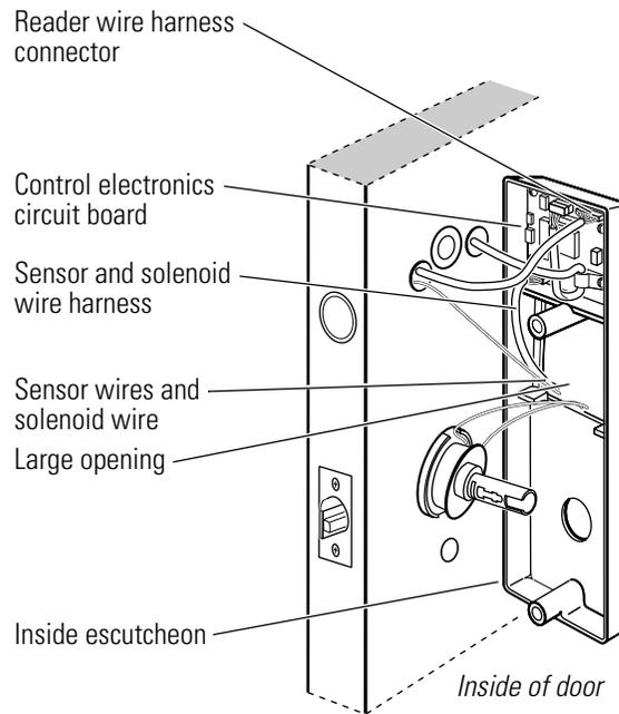
**Figure 4.5** Loosening the escutcheon and disconnecting the connections
