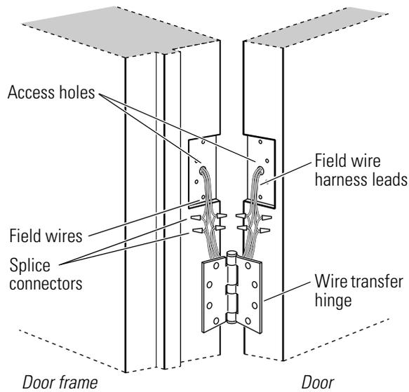
**Figure 4.10** Installing the wire transfer hinge
