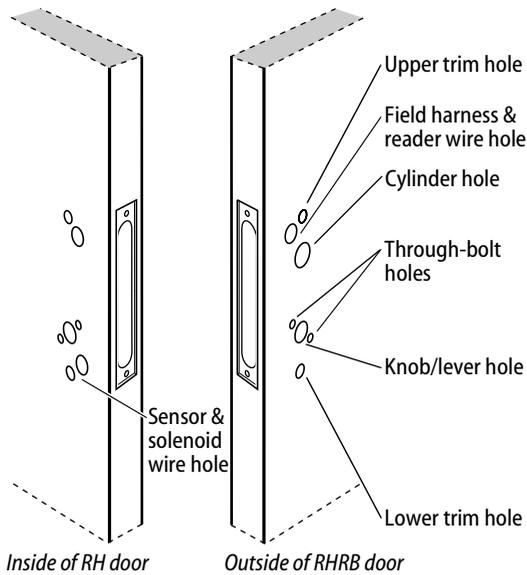
Figure 4a Drilling the RH and RHRB holes
