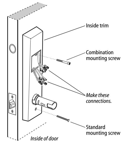
Figure 16 Securing the through-bolt trim and completing connections
