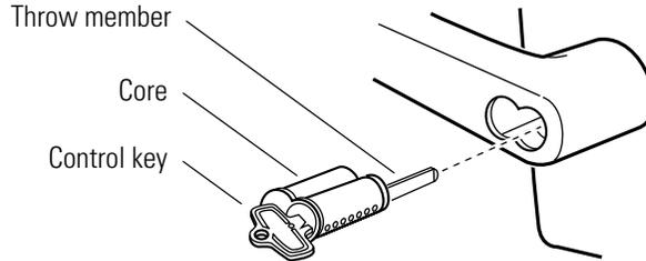
**Figure 4.1** Removing the core and throw member (lever shown)
