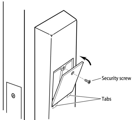
Figure 17 Installing the access door
