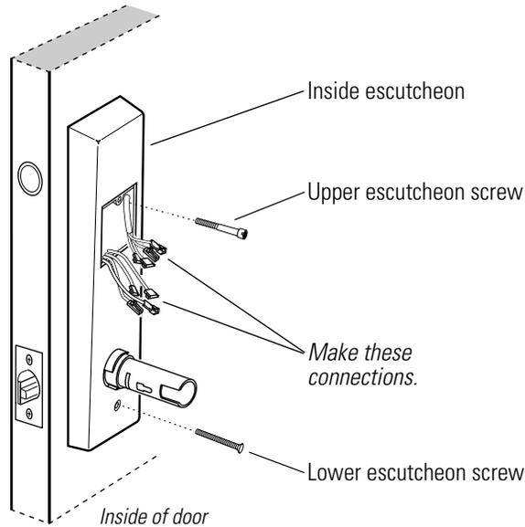
**Figure 4.17** Securing the through-bolt escutcheon and completing connections
