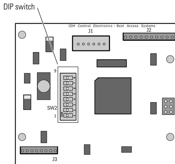
**Figure 2.6** Location of the DIP switch on the control electronics circuit board
