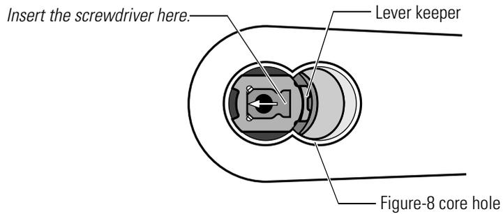
**Figure 4.2** Removing the keyed lever/knob (lever shown)
