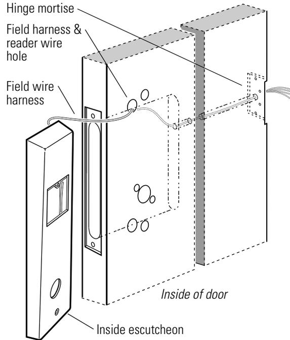
**Figure 3.13** Pulling the field wire harness through the door
