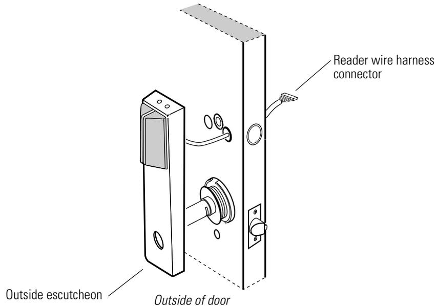
**Figure 4.6** Removing the outside escutcheon from the door
