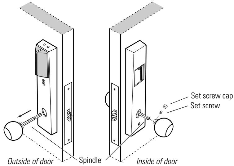
**Figure 3.2** Removing the knobs
