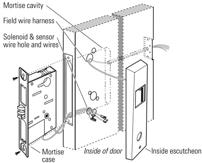
**Figure 3.15** Reinstalling the mortise case
