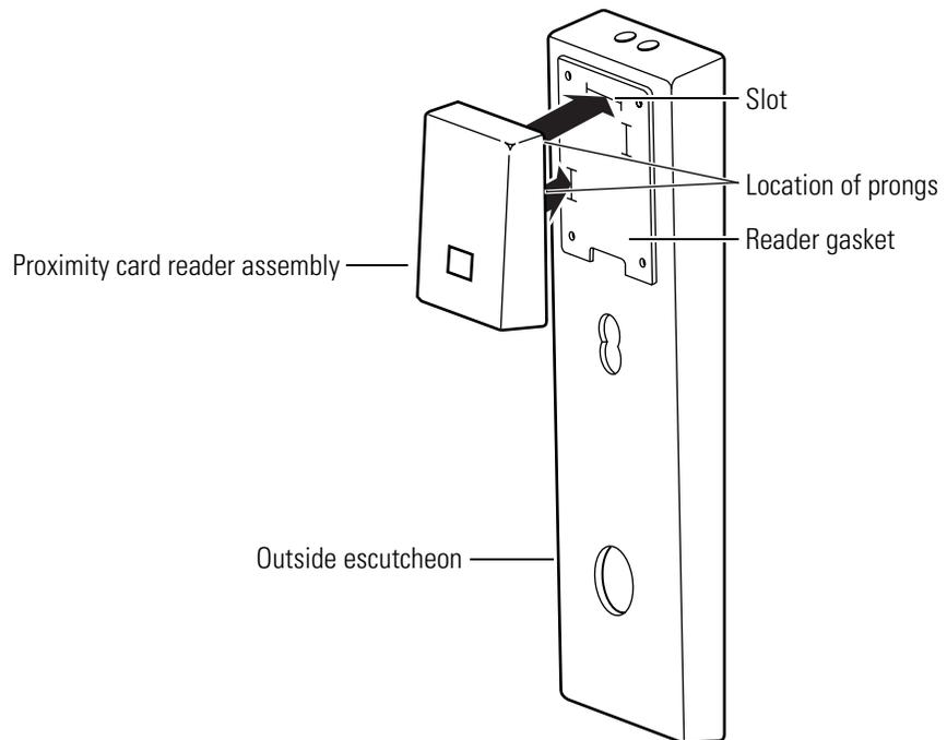
**Figure 5.6** Removing and replacing the proximity card reader
