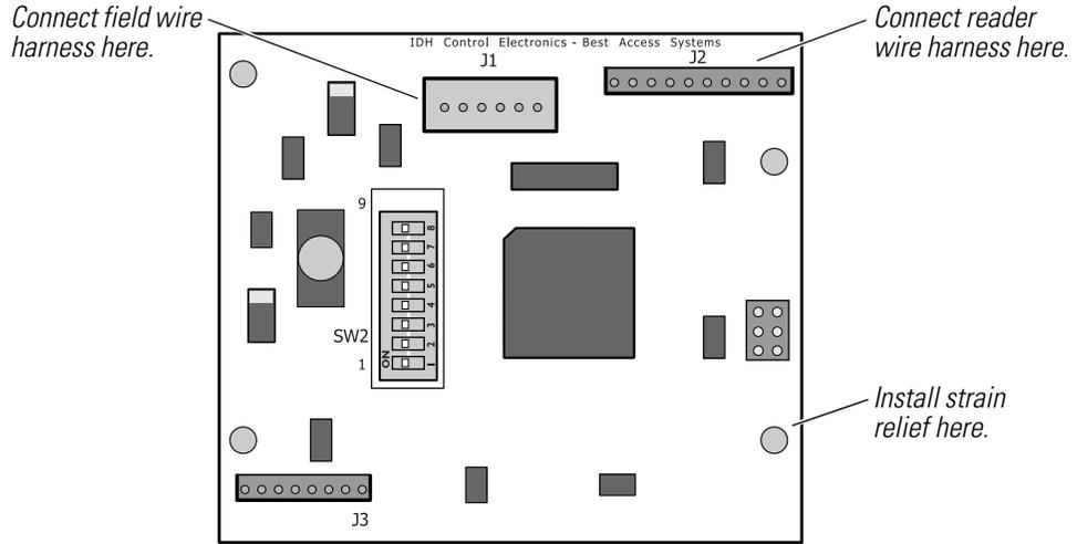
**Figure 5.3** Connecting the wire harnesses to the control electronics circuit board
