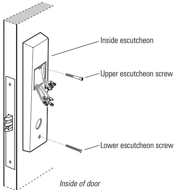
**Figure 3.5** Removing the inside escutcheon
