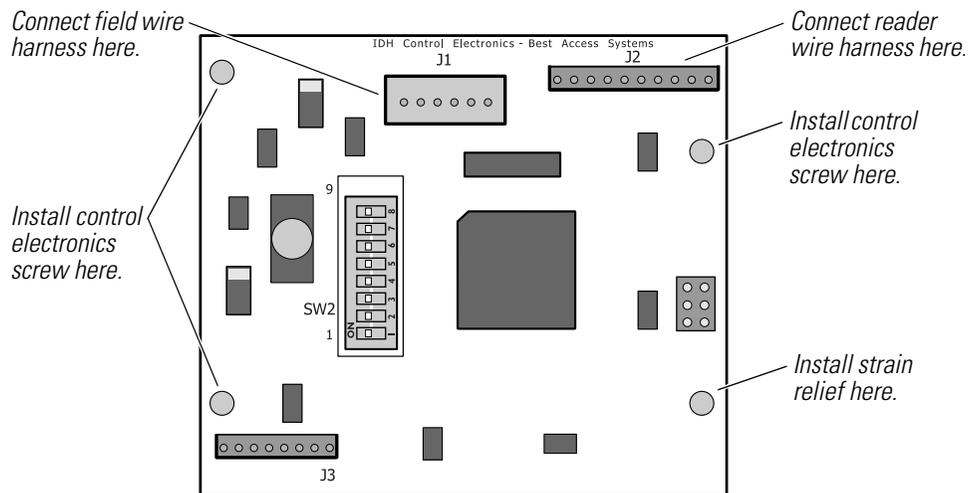
**Figure 5.4** Installing the screws for the control electronics circuit board
