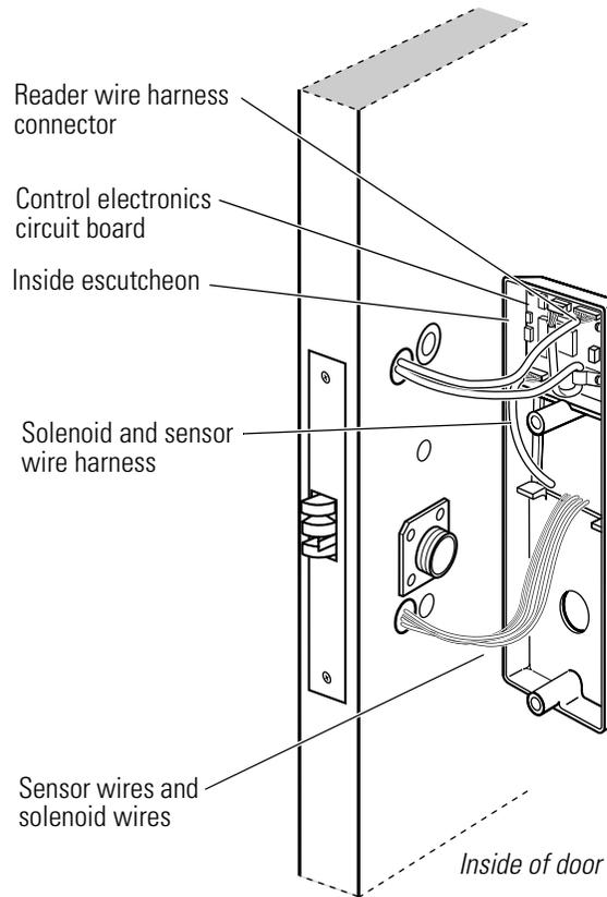
**Figure 3.6** Disconnecting the wire harnesses
