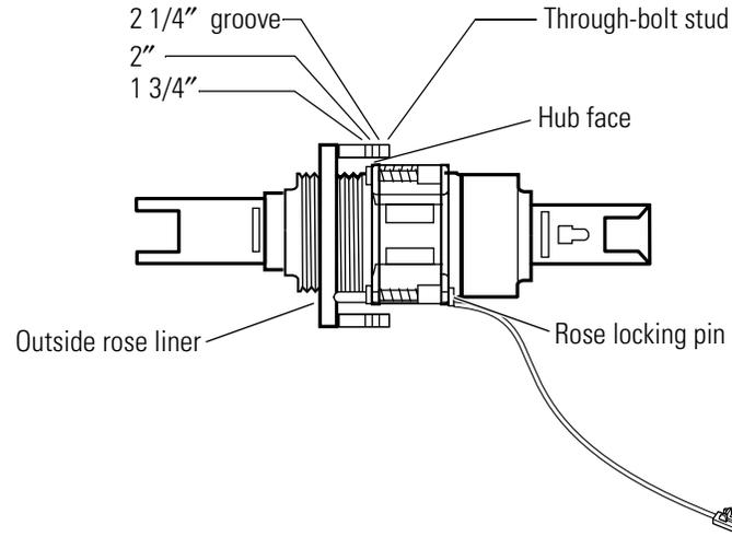
**Figure 4.11** Adjusting the outside liner for the door thickness
