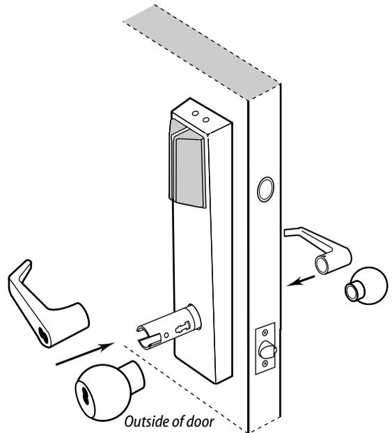
Figure 17 Installing the knobs/levers
