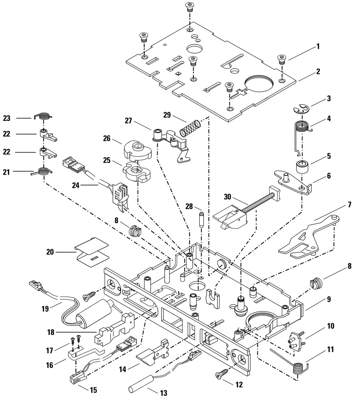
**Figure 2.7** Mortise case exploded diagram (EEU function shown)
