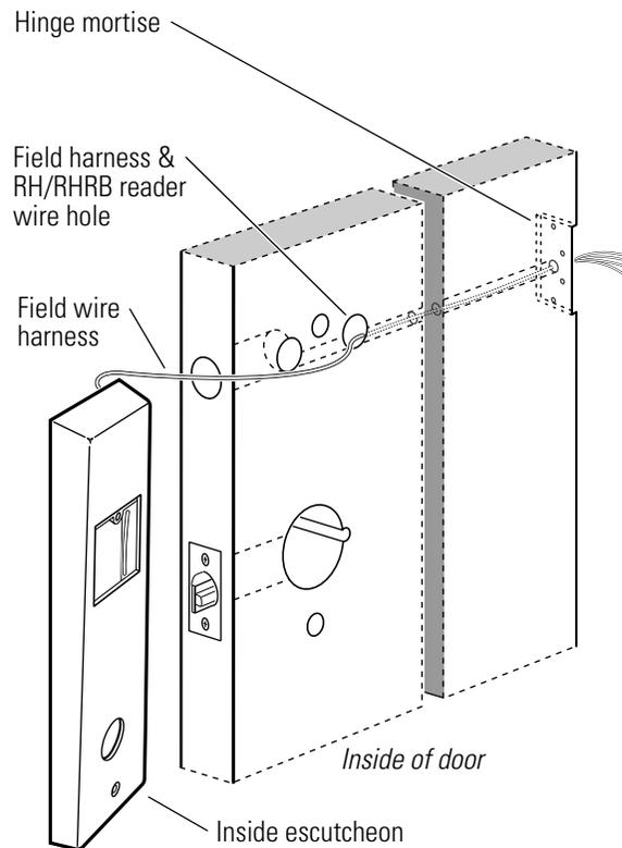
**Figure 4.9** Pulling the field wire harness through the door
