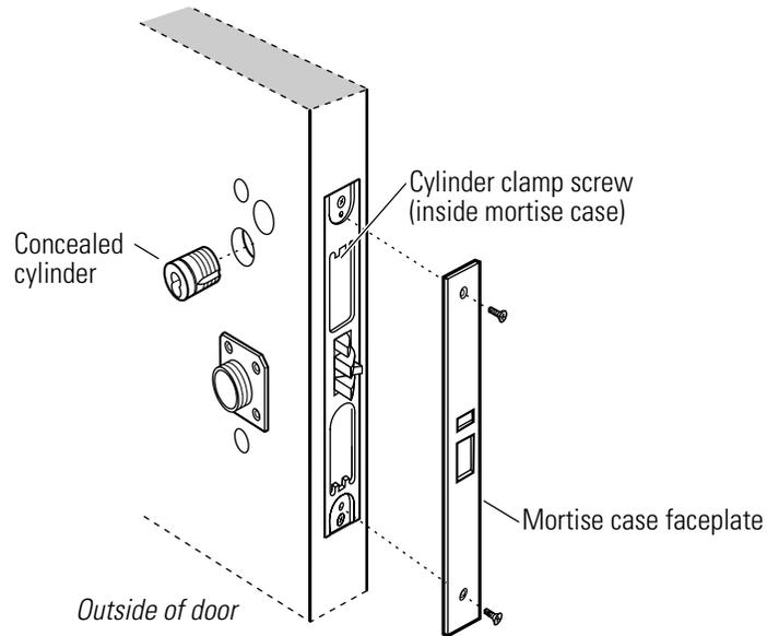
**Figure 3.9** Removing the mortise case faceplate and cylinder
