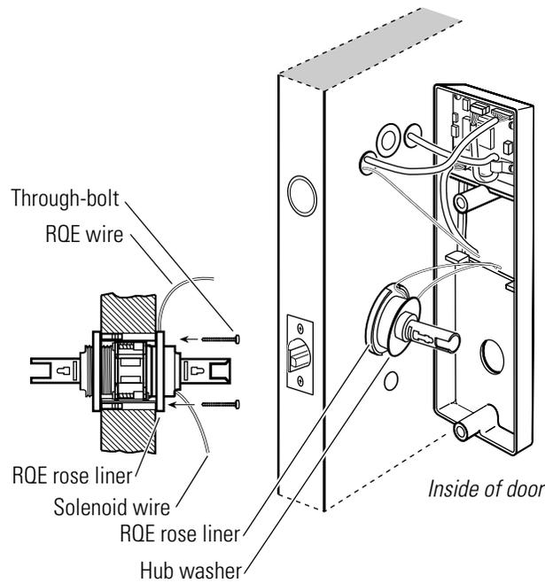
**Figure 4.13** Reinstalling the through-bolts and RQE rose liner
