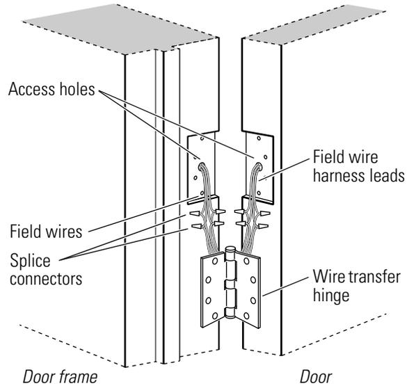
**Figure 4.8** Removing the field wire harness
