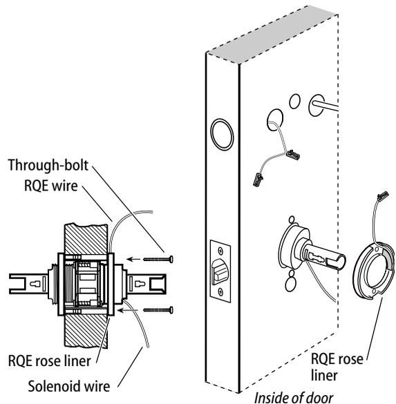
Figure 13 Installing the through-bolts and RQE rose liner
