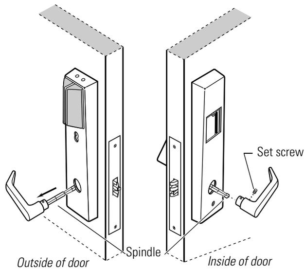
**Figure 3.3** Removing the levers
