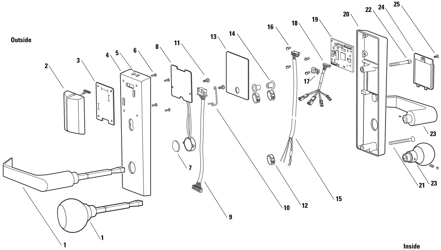
Figure 2.4 Magnetic stripe swipe card reader and trim exploded diagram
