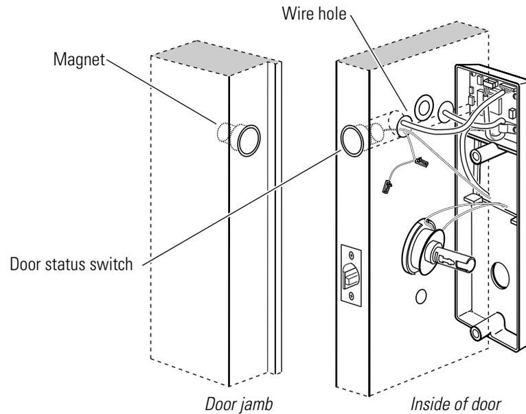
**Figure 4.23** Removing and reinstalling the door status switch and magnet assembly
