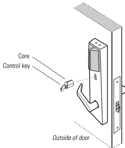
**Figure 3.24** Reinstalling the core
