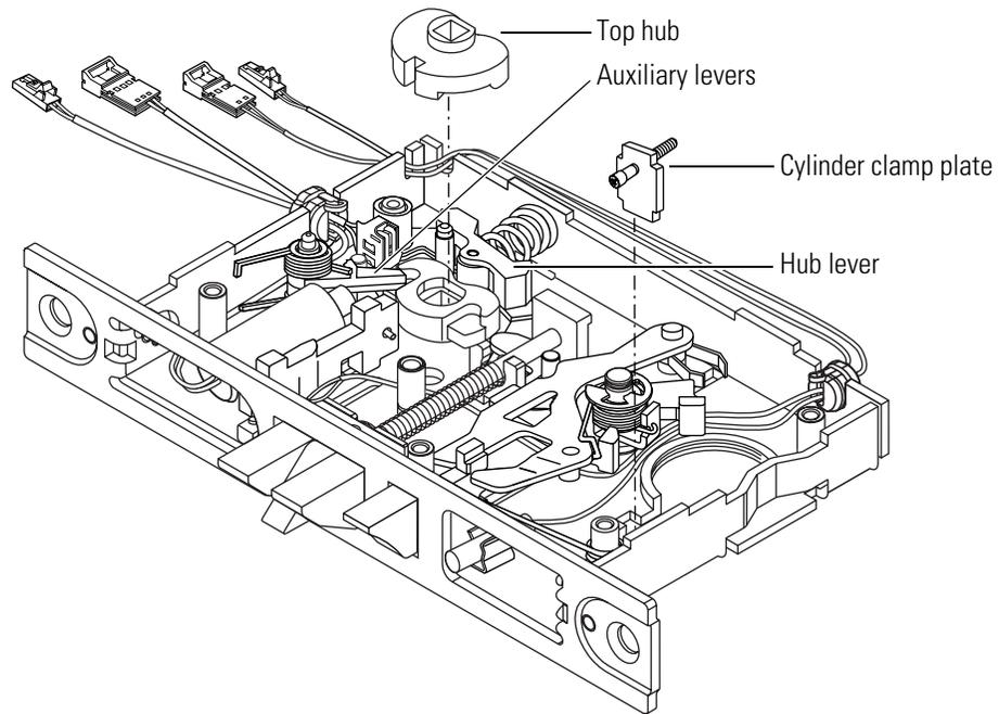
**Figure 3.31** Turning over the hubs and cylinder clamp plate (LHRB orientation shown)
