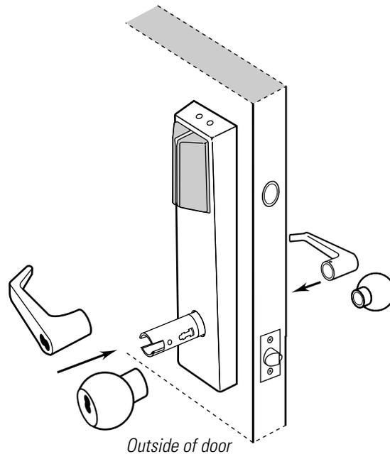
**Figure 4.18** Reinstalling the levers/knobs
