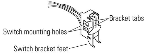
**Figure 3.30** Assembled RQE switch assembly
