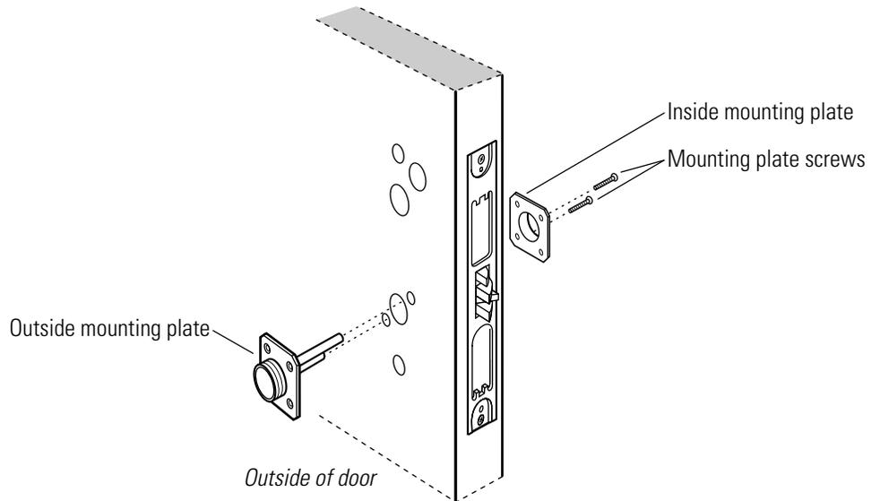
**Figure 3.10** Removing the mounting plates
