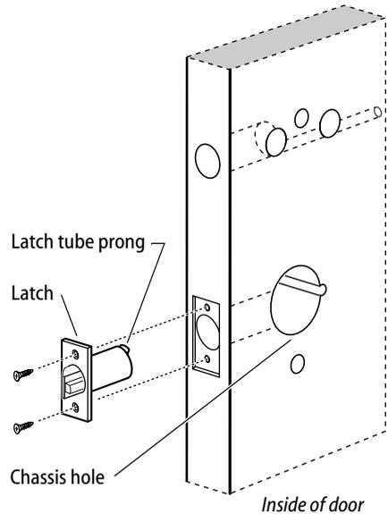
Figure 5 Installing the latch in the door
