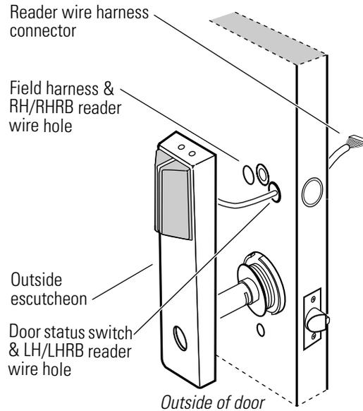
**Figure 4.15** Feeding the reader wire harness connector through the wire hole
