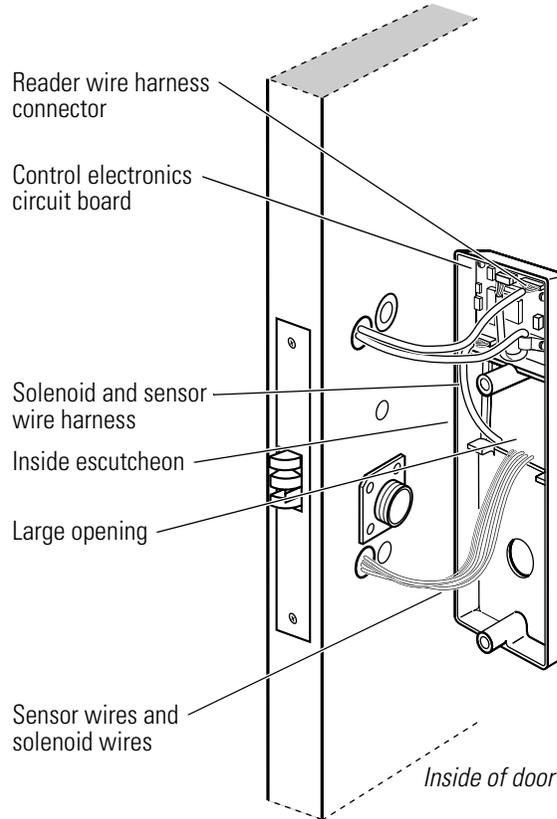
**Figure 3.20** Connecting the reader wire harness to the control electronics circuit board
