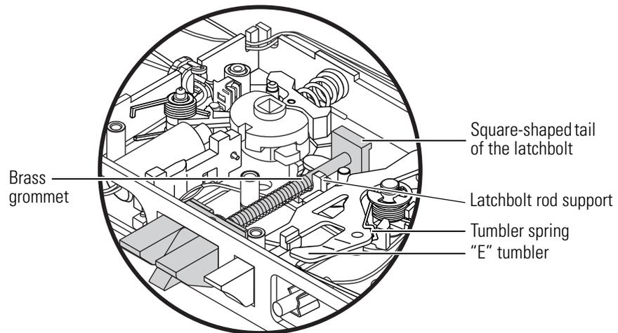
**Figure 3.35** Turning over the latchbolt (closeup, LHRB orientation shown)
