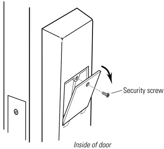
**Figure 3.4** Removing the access door
