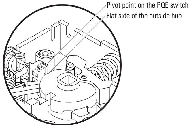
**Figure 3.32** RQE switch and hub orientation (closeup)
