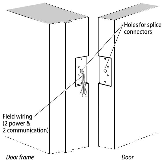
Figure 4 Preparing for the wire transfer hinge
