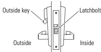
**Figure 2.1** Understanding mortise function drawings
