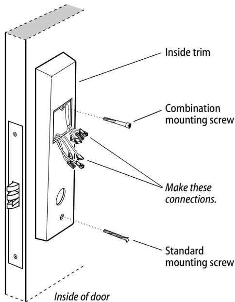
Figure 14 Securing the through-bolt trim and completing connections
