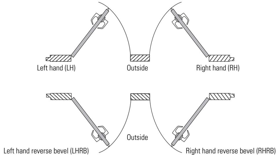
**Figure 3.26** Explanation of the hand and bevel of the door
