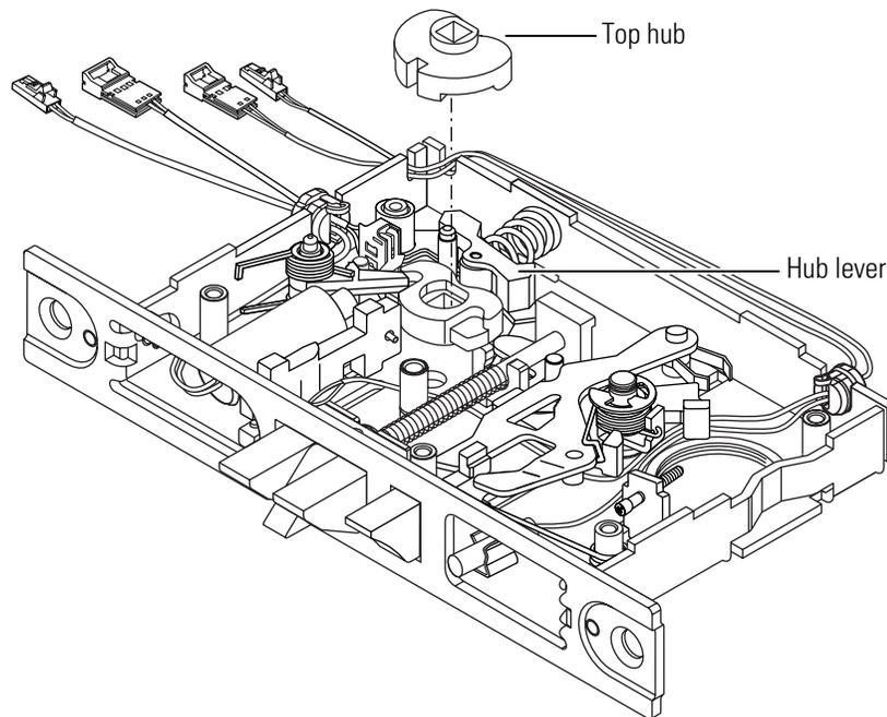
**Figure 3.28** Turning over the hubs (LHRB orientation shown)
