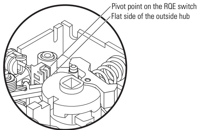
**Figure 3.38** RQE switch and hub orientation (closeup)
