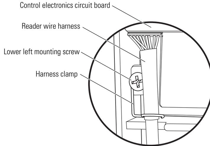
**Figure 5.2** Removing the harness clamp
