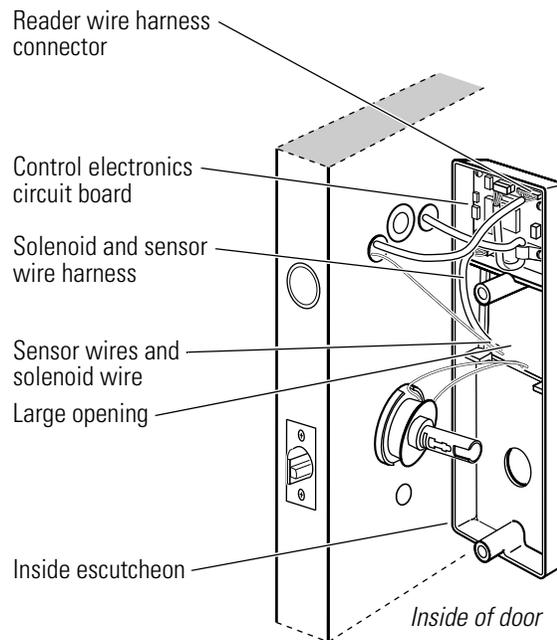
**Figure 5.1** Disconnecting and connecting the reader wire harness (cylindrical lock shown)
