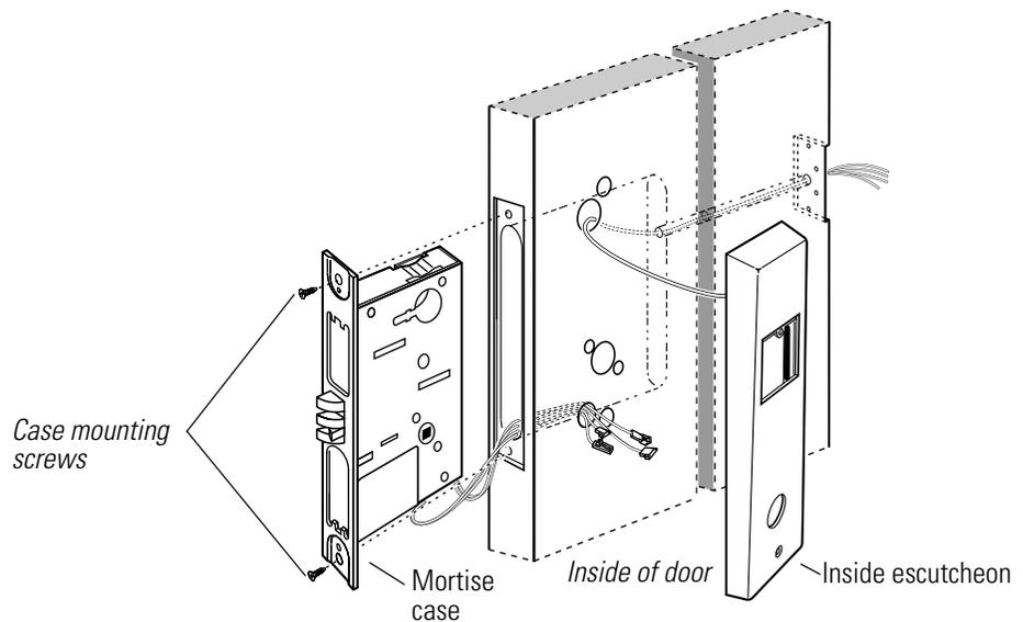
**Figure 3.11** Removing the mortise case
