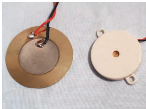
Fig.5. A ceramic resonator (left) and a cased resonator (right).
