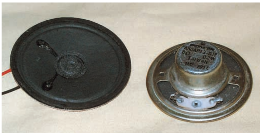
Fig.1. Miniature loudspeakers, such as those shown here, normally lack a built-in mounting bracket.
