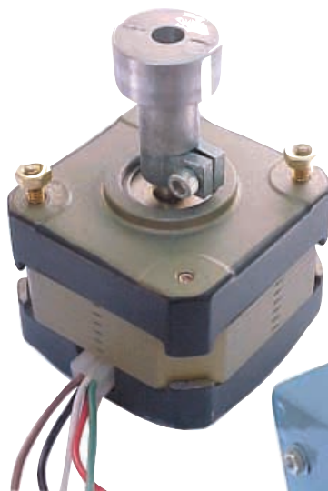
Prototype 12V four-phase unipolar stepper motor from an old 5 1/4 in. disk drive (circa 1982).
