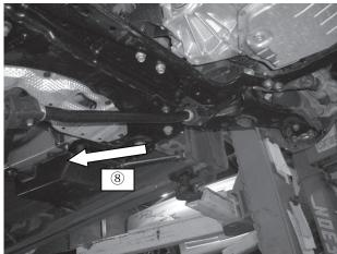
8.) Remove the sway bar from the driver side area.
