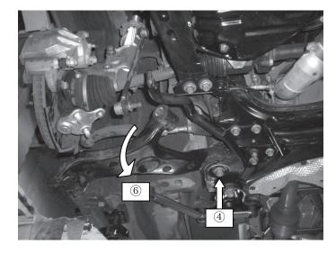
6.) Pivot the lower arm unit towards the rear of the vehicle by using the bolt loosened in step 4 as an axis point. This is to give enough space to remove the sway bar.
