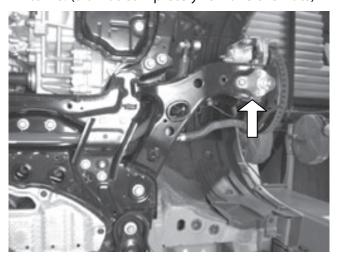
5.) Remove the 2 nuts and 1 bolt located on the lower left suspension knuckle.
