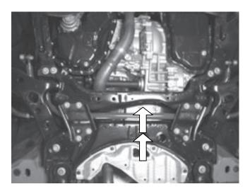
6.) Remove 1 bolt and 4 nuts holding the transmission mount.
