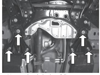
4.) Loosen the 6 bolts three full turns. (Do not completely remove the nuts)
