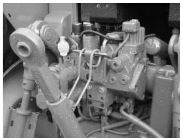
Figure 4: Old Style Stack Valve
