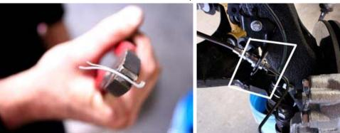
26. Remove the ABS line from behind the shock tower. Use supplied adell clamps to guide line across the Upper Control Arm, do the same with the clamps on the spindle using supplied bolts.
