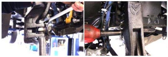
18. Rotate outer tie rods 180 degrees, this will now allow you to install the tie rod ends from the top of the steering arm.
