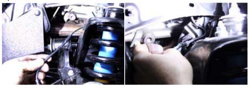
21. Remove bracket from upper control arm and discard, then remove ABS bracket from brake line bracket and discard
