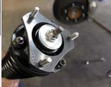
15. Reinstall the strut assembly. Leave the three upper strut mounting nuts loose. Raise the lower control arm and install the lower strut mounting bolt and nut. Use a floor jack to raise the lower arm up in order to get the lower ball joint bolts installed. Be sure to use thread locker on the lower ball joint bolts. Tighten all bolts to factory spec.
