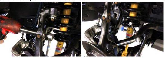
6. Remove the unit bearing, then discard backing plate & dust shield.
