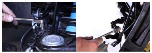
22. Bend the tab on the brake line bracket, then attach brake line bracket to the new spindle using the supplied hardware.
