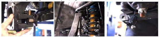
17. Attach lower ball joint / steering stop plate to the new spindle, tighten supplied 5/8"x3 ¼" bolts
