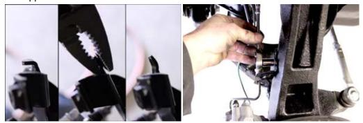
23. Remove stock brake line at the frame & caliper, then install new one. We suggest installing on frame side first, to let fluid bleed through the new line, then attach on caliper side.
