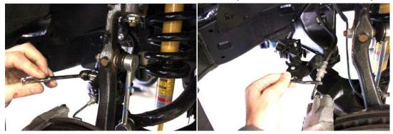
3. Remove brake caliper, then support it, do not allow it to hang from the brake hose.
