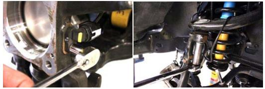
10. Remove bolts from lower ball joint / steering stop plate, then break upper ball joint loose by hitting the side of the spindle, do not hit the thread, remove spindle.
