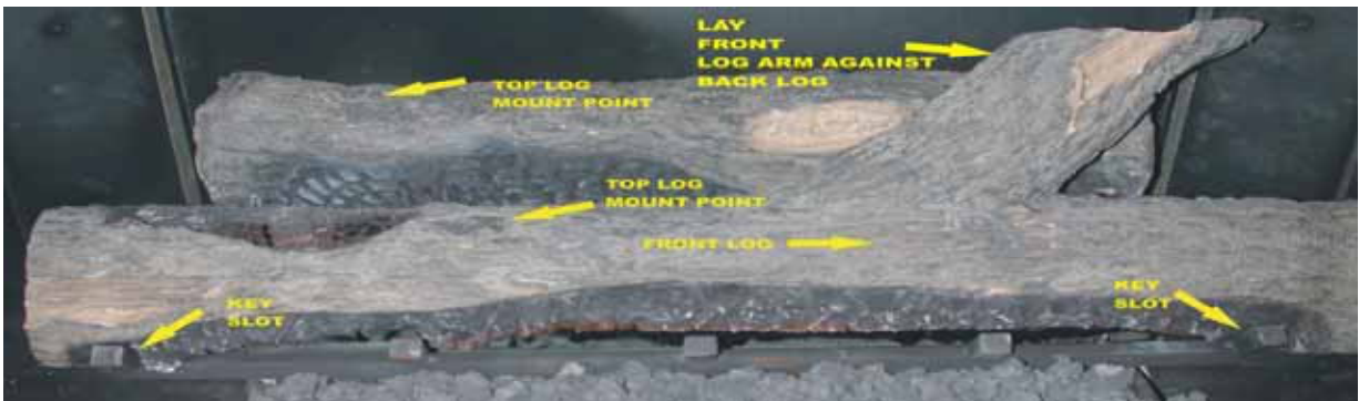
FIGURE 5b: FRONT LOG PLACEMENT
