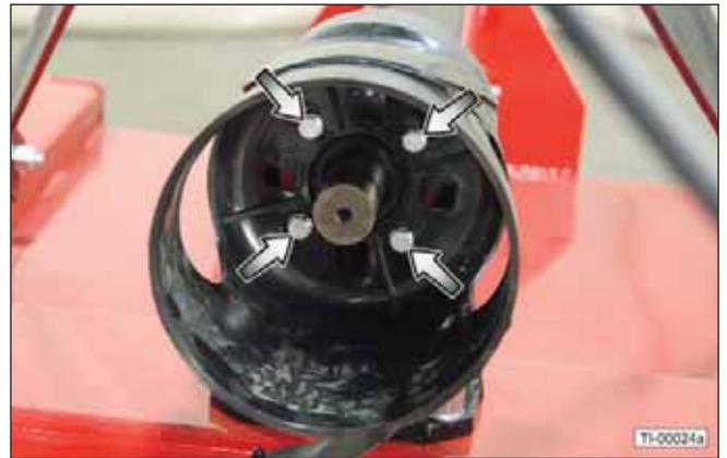
9. Separate the two halves of the driveline.
