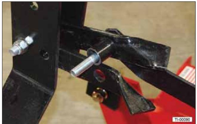
5. Tighten the bolt sufficiently to eliminate side play, but still allow the break link to function.
