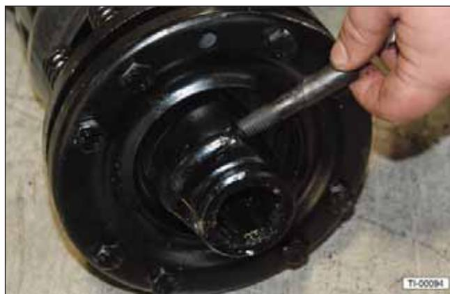
17. Line up the spline grooves and slide the slip clutch onto the gearbox input shaft until the retaining bolt hole aligns with the groove in the shaft.
