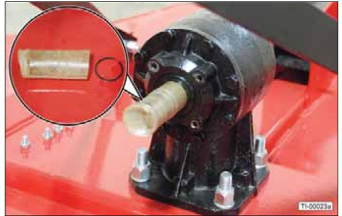
8. Position the driveline shield on the front of the gearbox and re-install the bolts.
