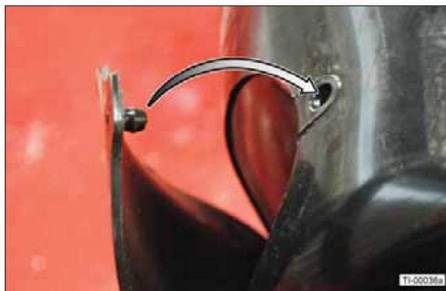
20. Slide the front driveline half over the rear half. Align the square rib on the mating halves to engage.
