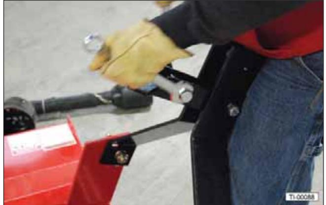
4. Position the back braces on the outside of the break link and reinstall the bolt. Be sure the spacer is in place.
