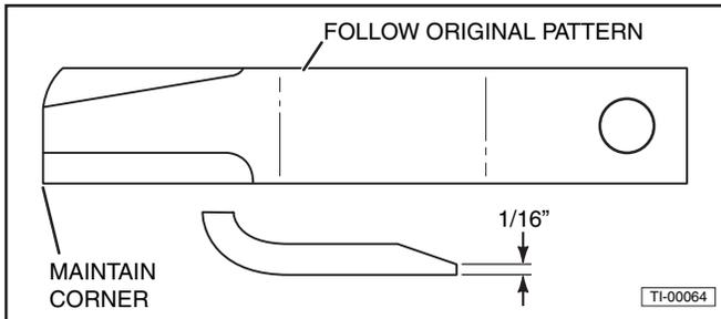
Replace the blades when worn more than 1/2" from the original edge. Always replace blades in pairs.
