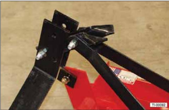
6. Remove the four 5/16-18 x 1/2" bolts from the front of the gearbox.
