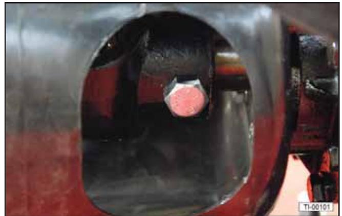
2. Rotate the driveline to align shear bolt with the access hole in the gearbox shield. Remove the damaged shear bolt.
