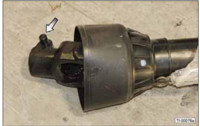
3. Push the driveline onto the tractor PTO shaft until the locking pin engages.
