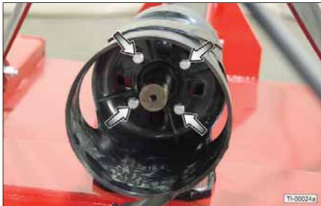
15. Separate the two halves of the driveline.
