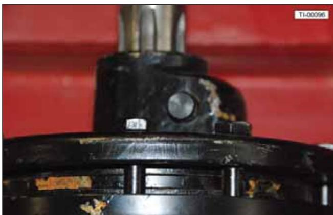
21. Apply grease to the zerk on the U-joint cross.
