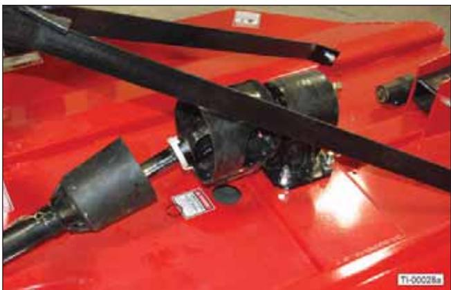
12. Install 1/2-13 x 3" Grade 2 shear bolt (11) and lock nut (12). Install the snap ring in the groove on the input shaft (shown by arrow).
