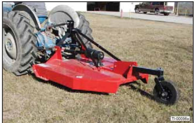
6. When turning, the angle between the tractor and rotary cutter should not be so great that a clattering of the U-joints occurs. Sharp turns can cause premature failure of the joints and put pressure on the tractor PTO shaft, and could cause extensive mechanical damage to the rotary cutter and tractor.
