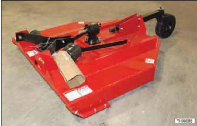
2. Cut the wires holding the driveline parts to the A-frame. Set the driveline aside for now.
