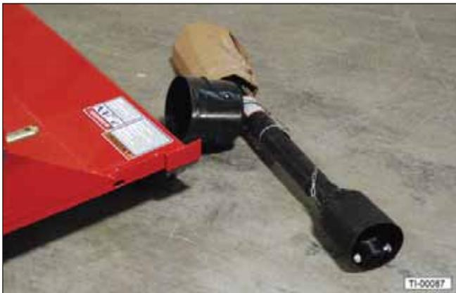
3. Stand the A-frame up and remove the 5/8-11 x 4-1/2" bolt, locknut, and spacer on the break link.
