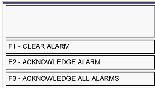
The Alarm History Screen displays all the acknowledged alarms with date and time. Using the arrow keys you can scroll through up to 50 previous alarm conditions. The Alarm History may be cleared with the Clear key.
