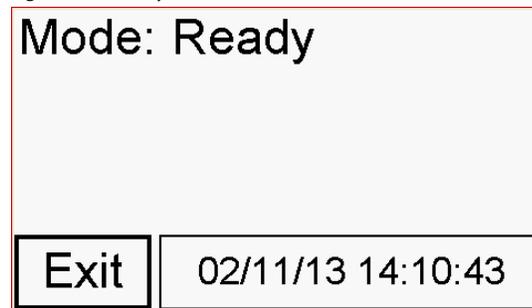
*Ready* mode ([Figure 13](#)) indicates the SyncPro II has not detected any software or hardware faults and is ready to start.
