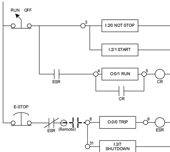
In both cases, the RUN output will follow the state of the START input, provided that all starting conditions are met. Note that in all cases, stopping the motor is done via the hardwired control circuit logic, and notification only is given to the SyncPro II.
