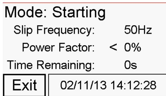
During the *Starting* mode ([Figure 14](#)), the motor slip frequency in Hz power factor in %, and time to a squirrel cage protection in seconds are displayed. The power factor value is accompanied by either a < or > symbol to indicate lagging or leading power factor. Typical power factor readings during starting are lagging. If leading power factor is displayed, please confirm voltage and current input connections for proper sequencing (e.g.  $V_{ab}$ ,  $I_c$ ).
