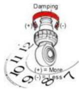
oil flow through the piston (more resistance to change) and less oil to bypass the piston through the hollow shaft and out the shaft. Left or counterclockwise allows less oil to push on the shim stack and more oil to bypass the piston (more resistance to change). You are looking up on the shock from the bottom of the shock to determine which way is clockwise as reference.
