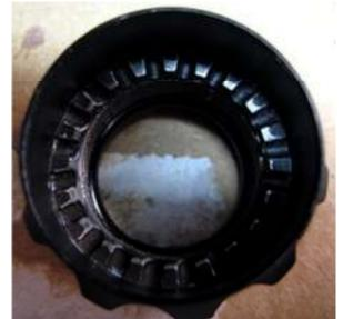
going up (#2) and you still keep on cranking the "Detents" of the aluminum detent ring will get sheared off much sooner than you will wear down a solid steel shaft that is supported 1/8" from the end of the overhang of the shock shaft (#2).
