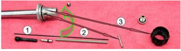
The shock shaft is hollow and assembly #1 is inserted inside of the shaft with the needle valve inside of the shaft. This needle valve lets oil from either side of the piston (top is rebound & bottom side is compression) bypass the shim stacks to the other side of the piston. This controls the percentage of oil goes through shim stacks which is how you adjust the shock for ride quality. Again: **The Springs Play No Part in This Suspension Other Than To Overcome Gravity!**
