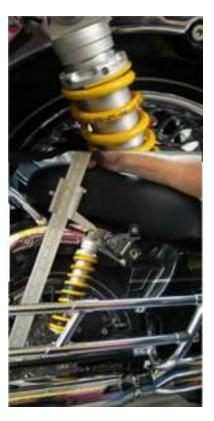
d. In this instance the total length from bolt from outside flat of the bolt to the bottom outside flat of the bolt with the wheel off of the ground was 349 mm. When the subject set on the bike and feet up on the boards and jack removed, the total sag was 28 mm as measuring from the
