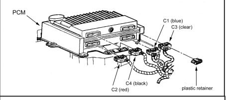
**DIAGRAM 3 - TWO-PLUG COMPUTERS -** The speed signal wire is located in connector C2 on vehicles equipped with this computer. Verify the pin number of the signal wire in chart "A" according the the vehicle model and year. The pin numbers are visible when the plastic retainer is removed from the back of the plug.
