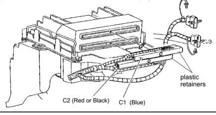
**NOTE:** Be extremely careful when disconnecting the plug from the computer; do not cock it to one side or pull on the wires in any way. Also note the color of the plug is only visible once the plug is removed from the computer.
