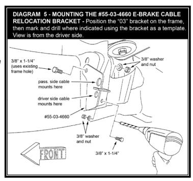
their respective holes in the frame and then reroute them so that they pass beneath the spring near the rear spring eye.
