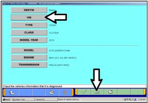
g. If the VIN or vehicle description displayed does not match the vehicle you are working on, click on the eraser icon at the bottom of the page.
