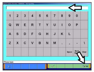
h. Click on the icon in the lower RH corner of the screen to have MUT-III automatically read the VIN. If a message appears saying that the VIN cannot be input automatically, manually type the 17 digit VIN into the VIN field at the top of the page.
