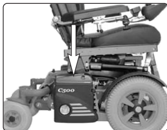
The charging fuse is located under the rear chassis cover
