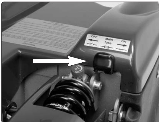
Main fuse in the ON position
