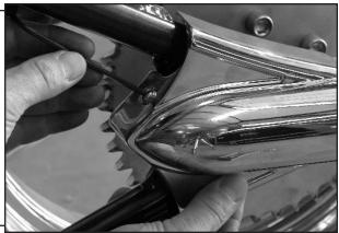
**STEP 4:** Now install the rear clamping tab using the hex head cap screw and lock washer provided in this kit. Apply Loctite 242 Blue to the threads of this screw and thread it into the cover along with the clamping tab as shown. The tab registers inside a notch in the cover and extends over the axle flange on the swing arm. Tighten this screw securely and repeat this step for each cover. your Torpedo axle covers are now fully installed.
