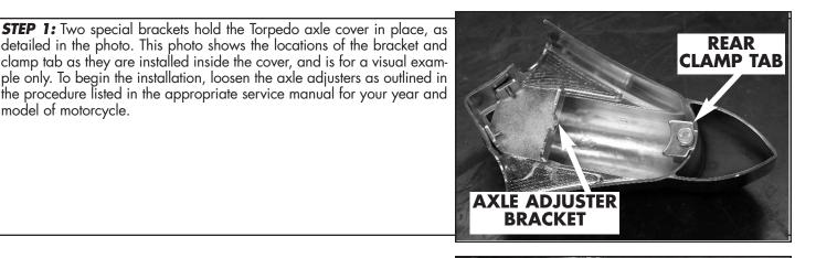
STEP 2: Install the axle adjuster bracket as shown. The bracket is clamped between the axle adjuster jam nut and the swingarm boss. Tighten the jam nut as specified in the procedure listed in the appropriate service manual for your year and model of motorcycle. Once these brackets have been installed on both sides of the swingarm it may also be necessary to verify rear wheel alignment and belt/chain tension as specified in your service manual.
