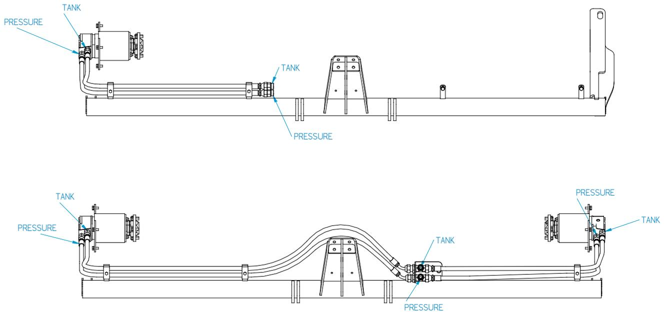
**Manual Angle:** Connect pressure line to female quick disconnect. Connect return line to male quick disconnect.
