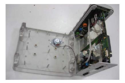
Figure 5-5 Disconnecting the Speaker Wires
