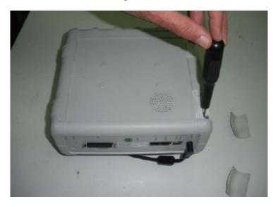
Figure 5-6 Removing the seven Retaining Screws
