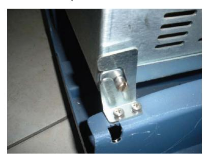
Figure 5-19 Isolator holder pins
