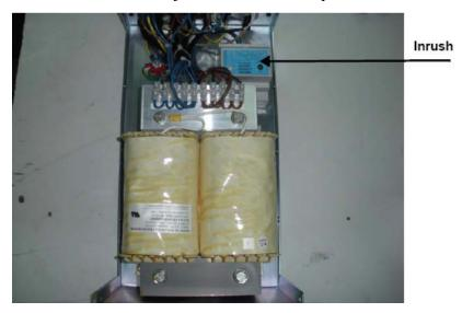
Figure 5-17 Inrush Current Limiter
