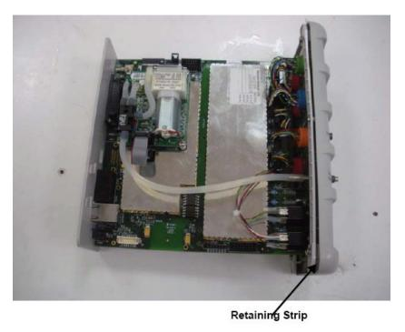
Figure 5-12 Retaining strip
