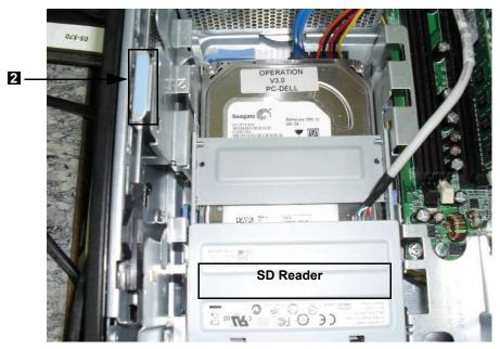
5. Squeeze two blue plastic clamps (3) simultaneously to unlock the hard disk. Push the hard disk backwards and pull out.
