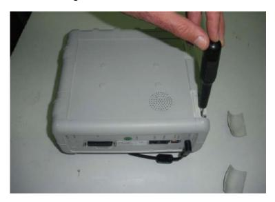
Figure 5-4 Detaching the Side Panel from the Top and Bottom Panels
