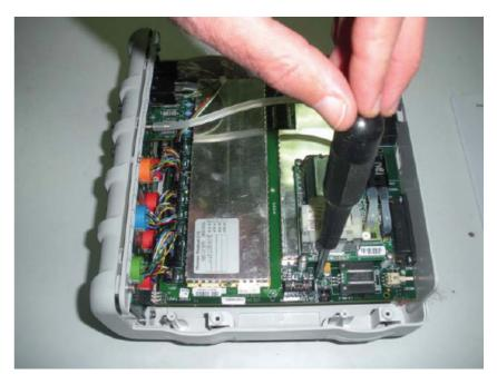
Figure 5-11 Relocating and securing the main board onto the right side panel
