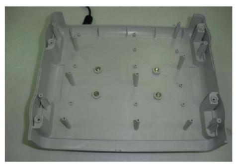
Figure 5-7 Right side panel after the CFE main board has been removed.
