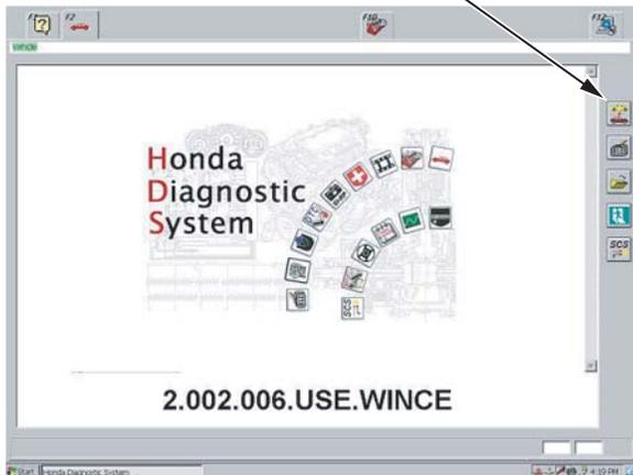
6. At the screen prompts, enter the VIN and the odometer reading, and then verify the correct date and time.
