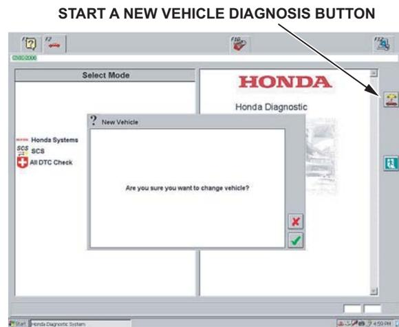
25. Manually enter the VIN and the odometer reading into the HDS. The HDS will ask you to confirm the VIN. When you select the green check mark to confirm the VIN, the HDS writes it into the replacement ECM/PCM.
