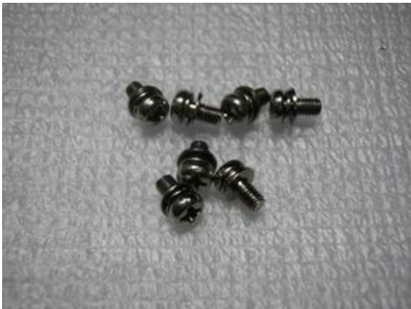
Review the seven piece screws (S05) and take off the main shield.
