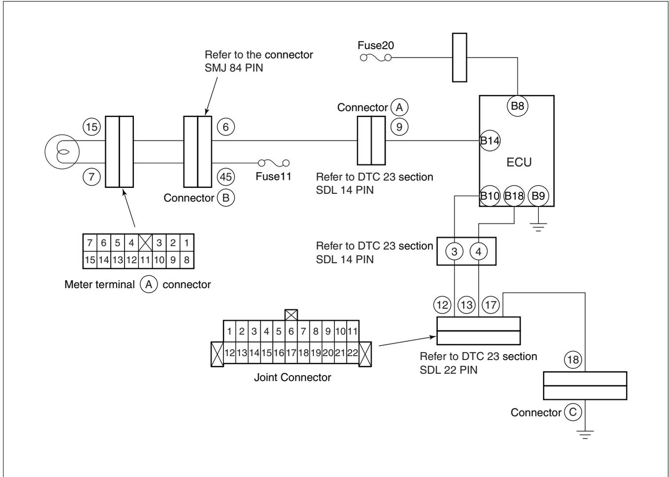
(2) The W/L lamp will not come on even when the starter SW is on.
