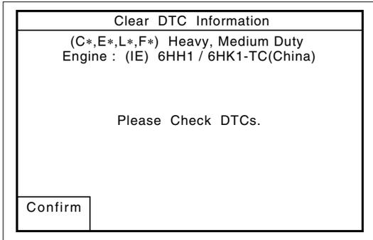
13. After the DTC number is cleared, check and confirm the DTC number.
