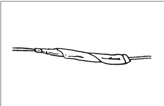
If the wire does not belong in a conduit or other harness covering, tape the wire again. Use a winding motion to cover the first piece of tape.
