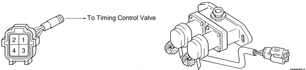
Timing Control Valve side connector
