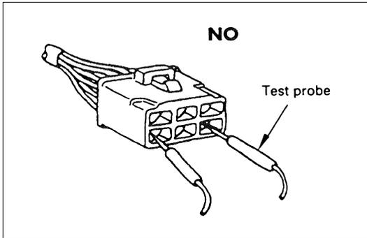
Never insert the circuit tester test probes into the connector open end to test the continuity. Broken or open connector terminals will result.
