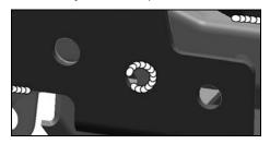
Once all welding is complete, spray paint entire Trackbar Brace and any bare metal on axle housing to prevent corrosion. All exposed metal must be completely covered.
