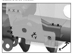
**HINT:** Be sure to include area on lower spring mount where it makes contact with Trackbar Brace. Also include back side of axle tube where Trackbar Brace wraps underneath.
