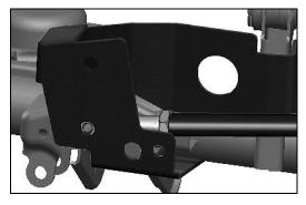
...or use the upper mounting hole if vehicle has a "drag link flip" or high-steering conversion. When track bar is installed in the upper hole, supplied steel sleeve must be installed in the lower hole using hardware provided.
