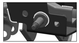
If you are not installing the optional steering stabilizer mount, plug weld Trackbar Brace to factory trackbar mounting bracket at location indicated by a "Y" in step 2.
