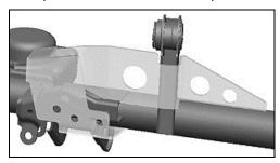
With Trackbar Brace in position, insert one M12 x 70mm Bolt (C) into original mounting hole as illustrated below. Secure bolt with original flag nut and temporarily tighten to hold the brace securely to the factory bracket.
