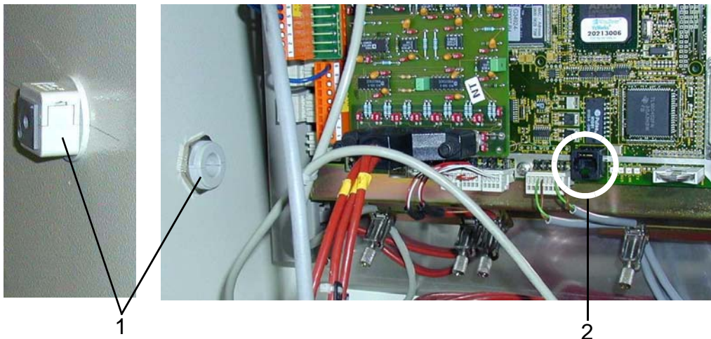
Fig. 1-1 Ethernet interface - Test system with Simcon controller
