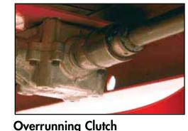
A greaseable overrunning clutch prevents beater backlash force when the PTO is disengaged, allowing the beaters to free wheel to a stop. This provides protection for the gearbox and spreader driveline.
