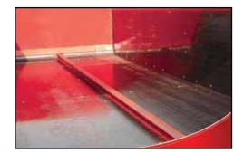
**Solid Poly Floor and Sides** The solid poly floor and sides reduce friction and promote self-cleaning to help prevent material buildup on the inside of the spreader.
