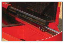
**Piggyback Hydraulic Cylinders** This unique cylinder design provides smooth and uniform travel through the entire stroke and rapid cylinder retraction when spreading is completed.
